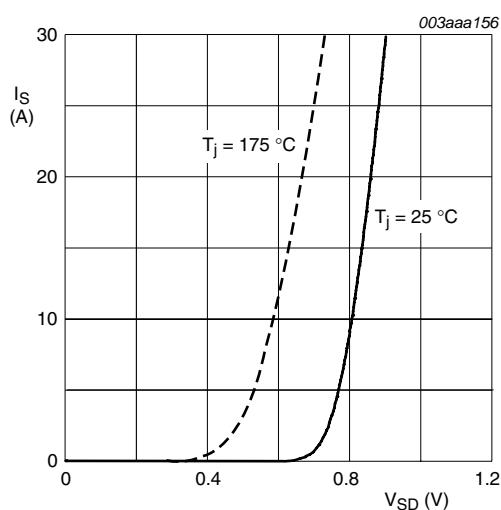
$T_j = 25^\circ C \text{ and } 175^\circ C; V_{GS} = 0V$
