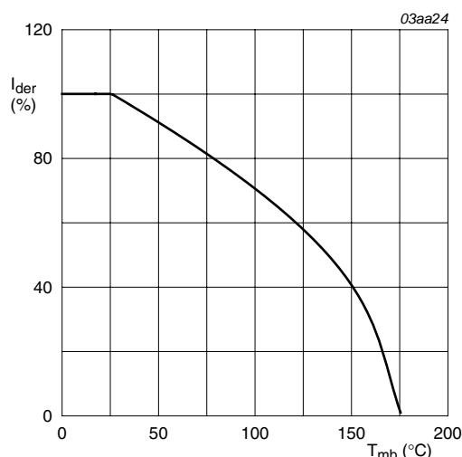
$$I_{der} = \frac{I_D}{I_{D(25^{\circ}\text{C})}} \times 100\%$$
