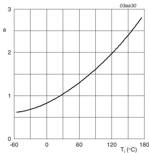
$$a = \frac{R_{DSon}}{R_{DSon}(25^\circ\text{C})}$$
