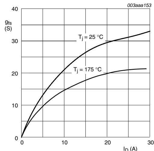
$T_j = 25^\circ\text{C}; V_{DS} > I_D \times R_{DSon}$
