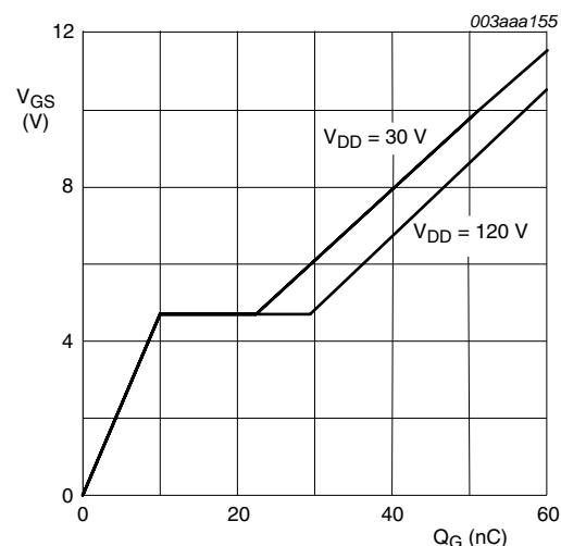
$I_D = 30 \text{ A}; V_{DS} = 30 \text{ V}$  and  $120 \text{ V}$
