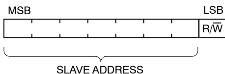
Figure 31. First Byte after START Procedure
