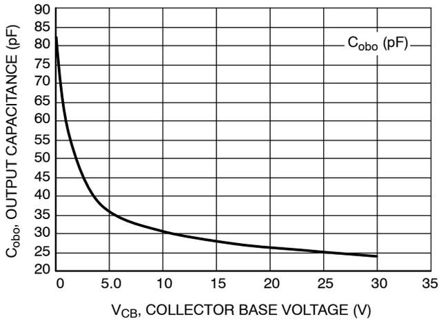
Figure 9. Output Capacitance
