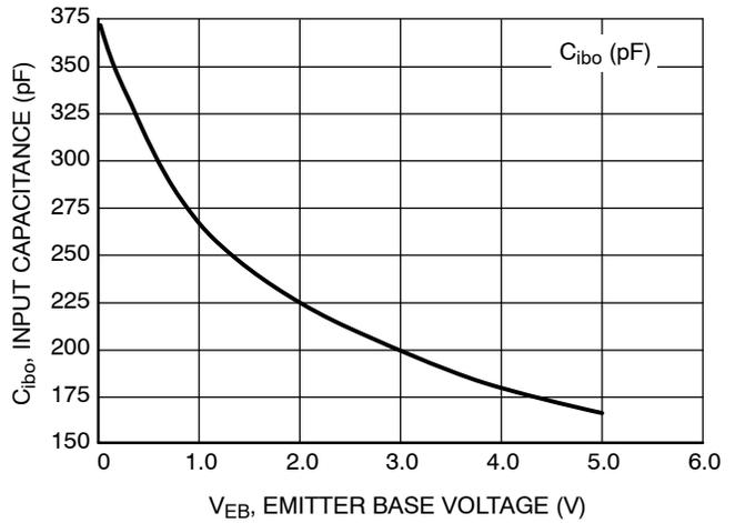
Figure 8. Input Capacitance
