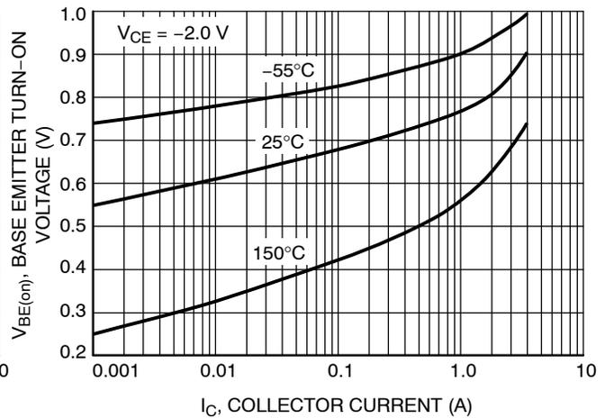
**Figure 6. Base Emitter Turn-On Voltage vs. Collector Current**
