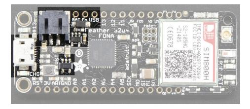
The above shows the Micro USB jack (left), Lipoly JST jack (top left), as well as the 3.3V regulator and changeover diode (just to the right of the JST jack) and the Lipoly charging circuitry (to the right of the Reset button). There's also a **CHG** LED, which will light up while the battery is charging. This LED might also flicker if the battery is not connected or when the cellular module is in action
