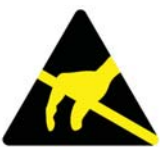
PESW-AA-11Y Warning of Static Sensitive Device
