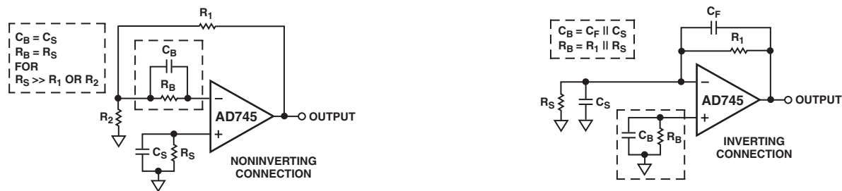
Figure 40. Optional External Components for Balancing Source Impedances
