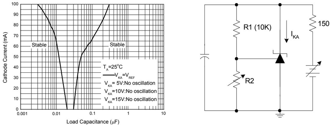
Figure 15. Stability Boundary Conditions vs. Load Capacitance
