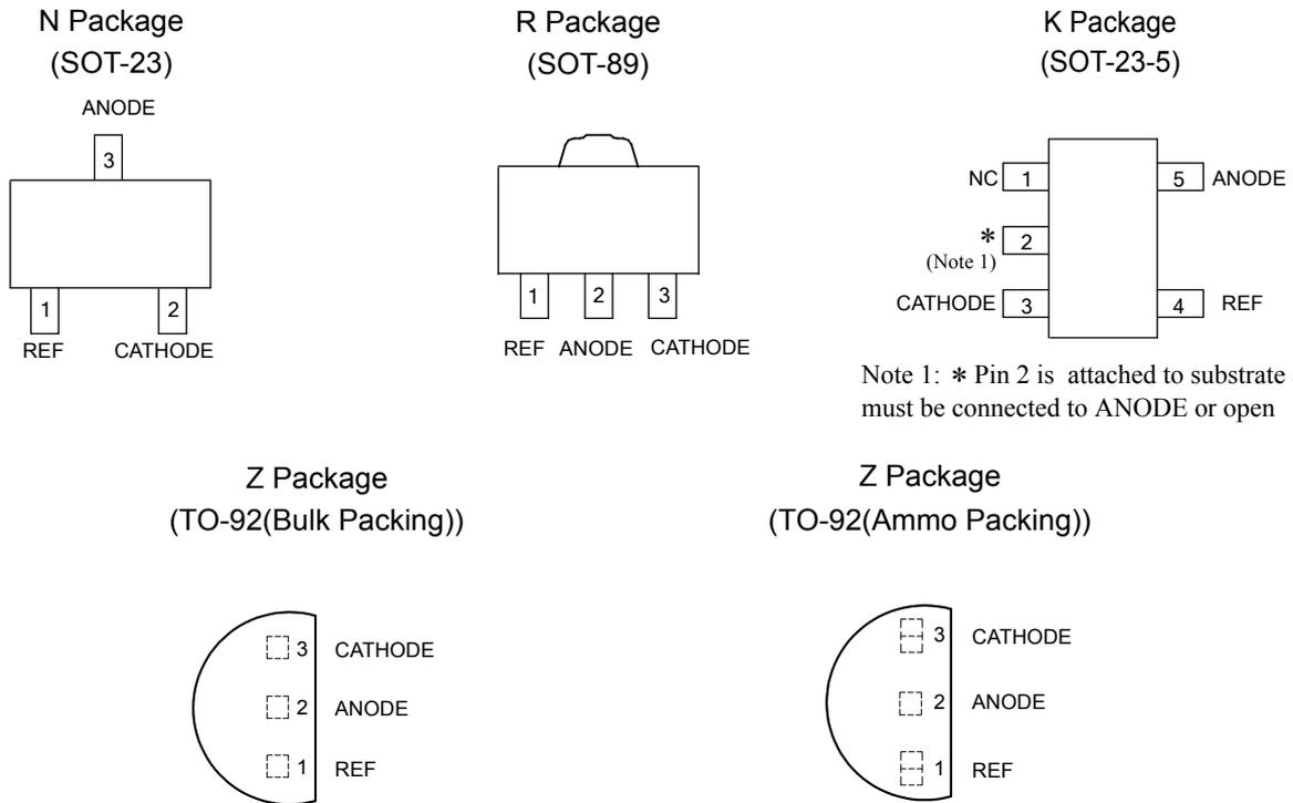
Figure 2. Pin Configuration of AS431 (Top View)
