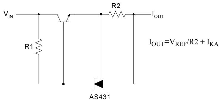
Figure 19. Current Source or Current Limit
