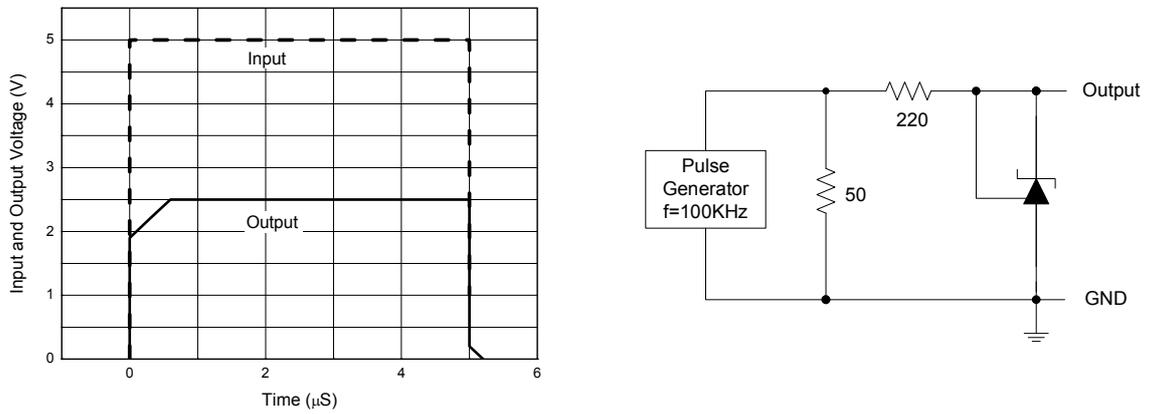
Figure 16. Pulse Response of Input and Output Voltage
