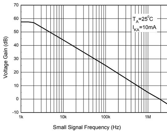
Figure 13. Small Signal Voltage Gain vs. Frequency
