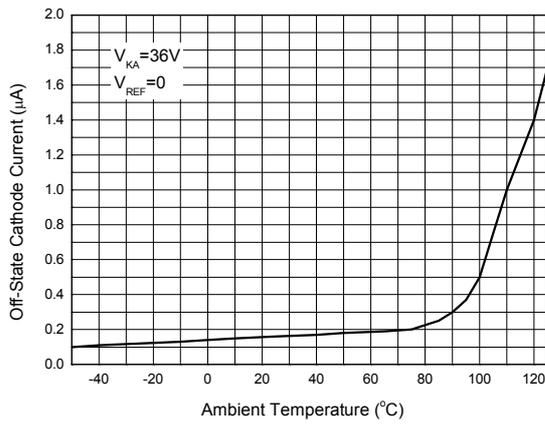
Figure 11. Off-State Cathode Current vs. Ambient Temperature
