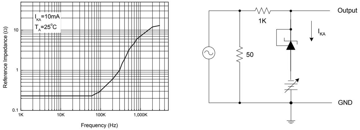
Figure 14. Reference Impedance vs. Frequency
