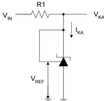
Figure 4. Test Circuit 4 for  $V_{KA} = V_{REF}$
