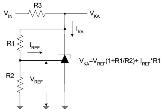
Figure 5. Test Circuit 5 for  $V_{KA} > V_{REF}$
