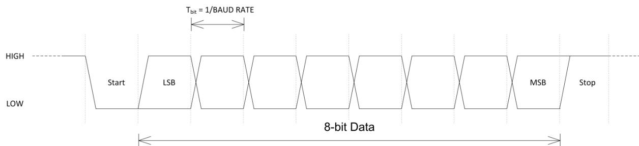
Figure 9-2: TTL Serial Timing Diagram
