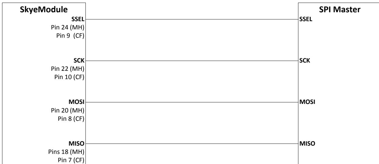
**Figure 9-3: SPI Connection Diagram**
