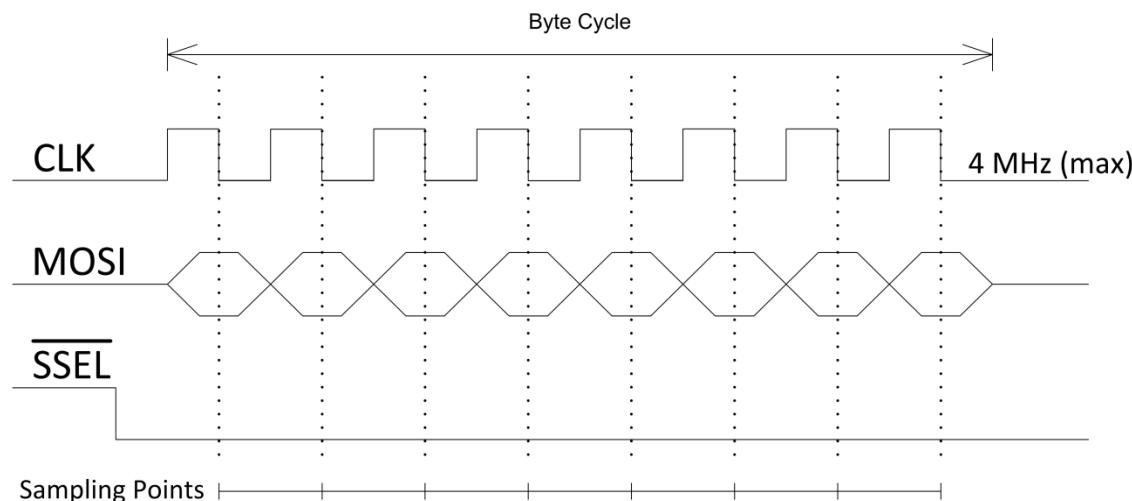
Figure 9-4: SPI Request Setup and Sample Timing
