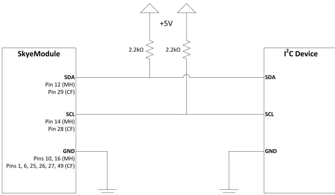
**Figure 9-8: I<sup>2</sup>C Connection Diagram**
