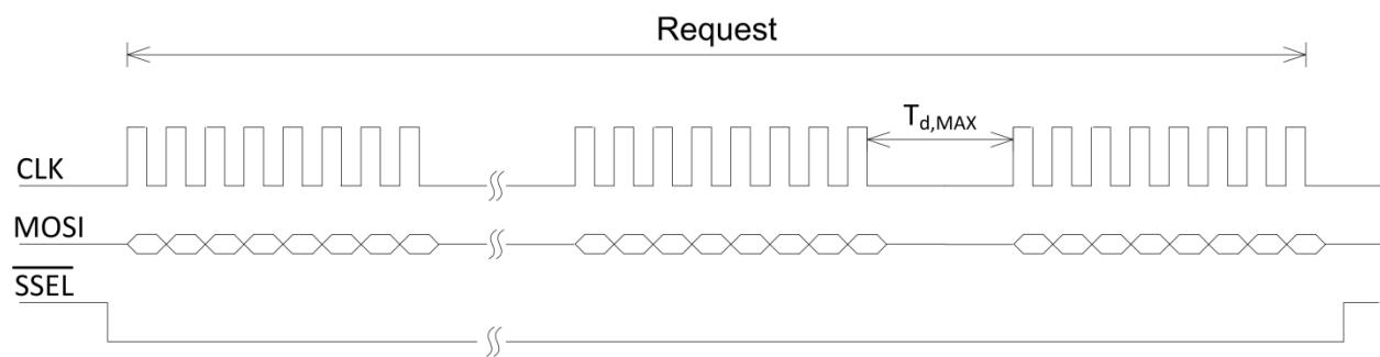
Figure 9-5: SPI Request Timing
