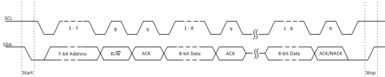
**Figure 9-9: I<sup>2</sup>C Timing Diagram**
