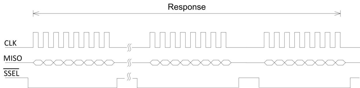
Figure 9-6: SPI Response Timing
