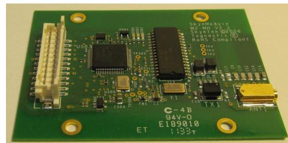
Figure 5-2: SkyeModule M2-MH
