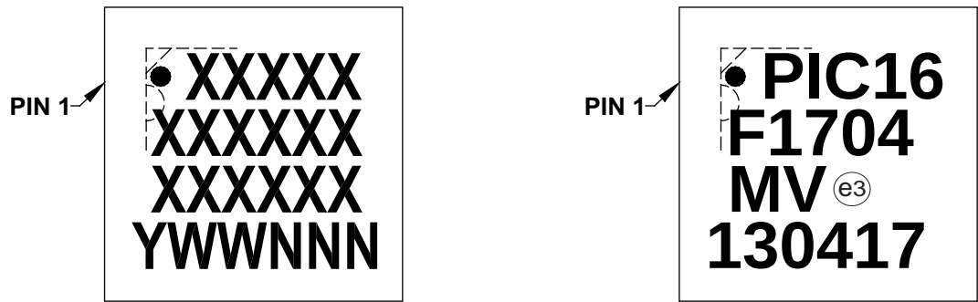
16-Lead QFN (4x4x0.9 mm)
