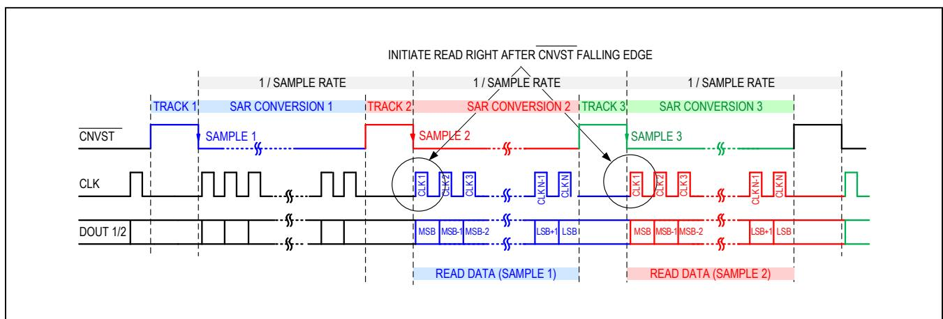
Figure 8. Reading Data After Falling Edge of  $\overline{\text{CNVST}}$
