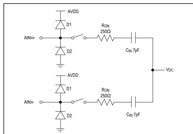
Figure 2. Simplified Model of Input Sampling Circuit
