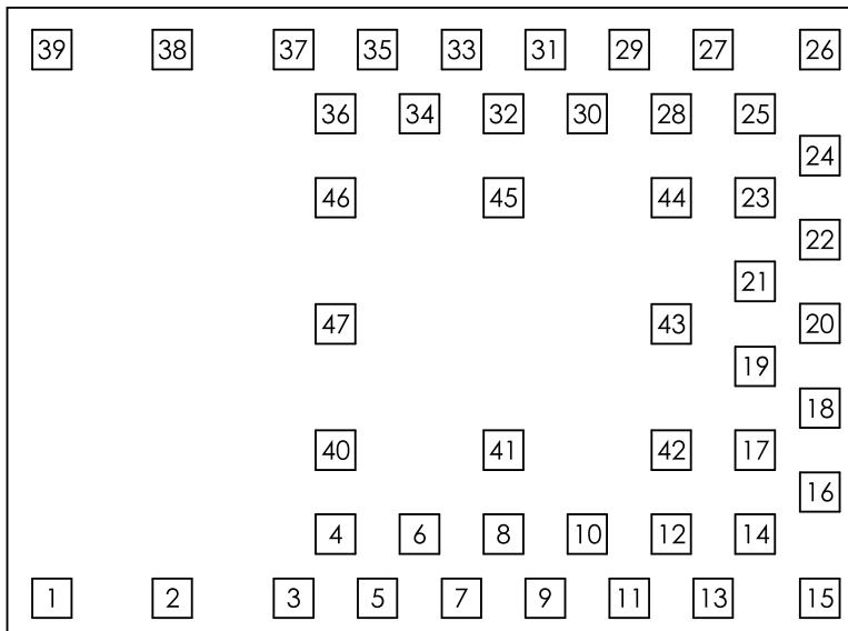
Figure 3 – BMD-350 Pin out (Top View)
