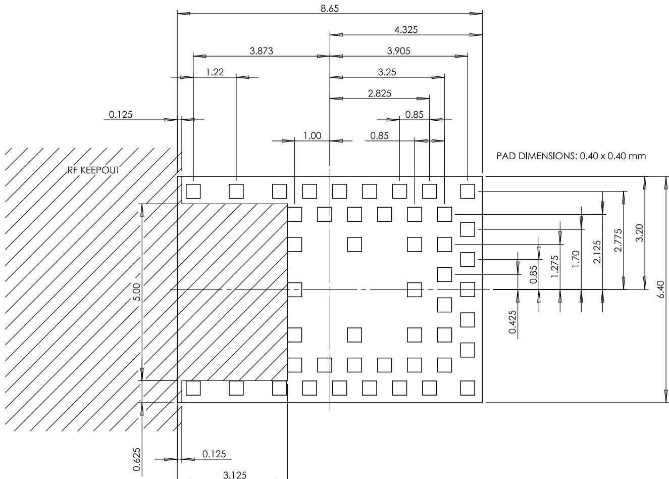
Figure 10 – BMD-350 Dimensions (Top View)
