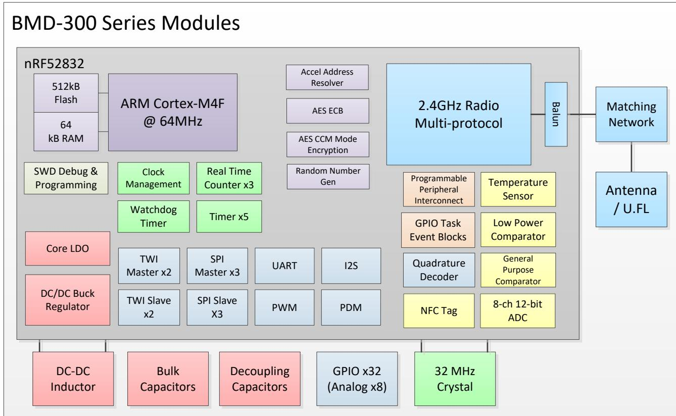
Figure 1 – Block Diagram
