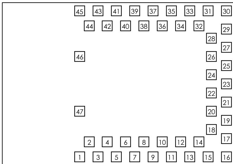
Figure 2 – BMD-300/301 Pin out (Top View)
