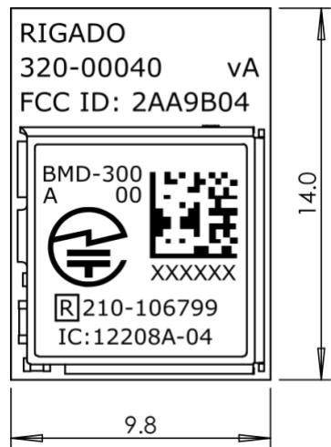
Figure 11 – BMD-300 Module Marking – Rev A
