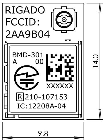
Figure 12 – BMD-301 Module Marking – Rev A
