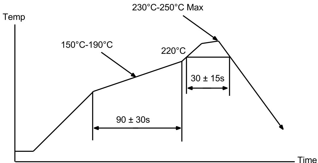
Figure 23 – Reflow Profile for Lead Free Solder
