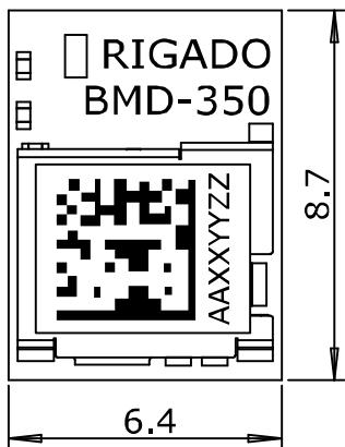
Figure 13 – BMD-350 Module Marking – Rev A
