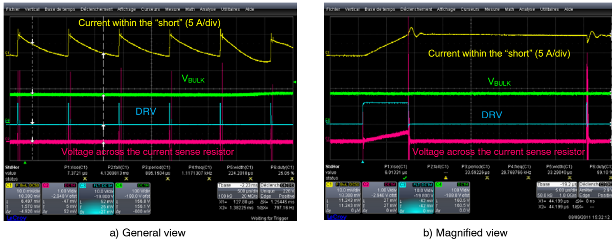
Figure 17. Shorting the Bypass Diode and the NTC
