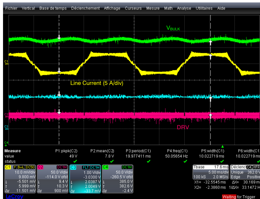
Figure 14. Over-Current Situation (85 V, 0.5 A Load Current)
