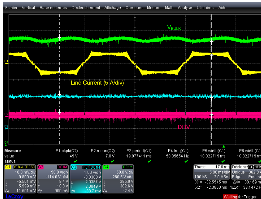
Figure 14. Over-Current Situation (85 V, 0.5 A Load Current)
