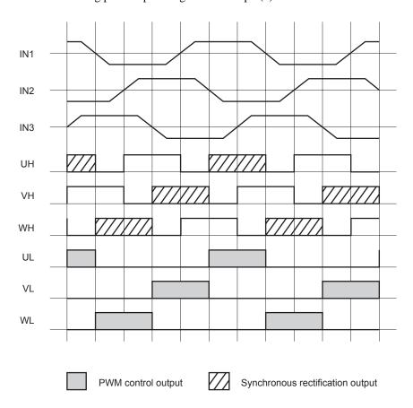
(4) When F/R="H" and the inverting phase input as against Hall input(1).
