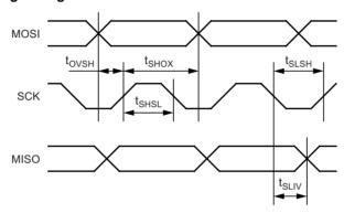
Table 23-8. Serial Programming Characteristics,  $T_A = -40^{\circ}\text{C}$  to +125°C,  $V_{CC} = 2.7 - 5.5\text{V}$  (Unless Otherwise Noted)
