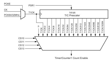
In the asynchronous clocking mode the clock selections are from PCK to PCK/16384 and stop, and in the synchronous clocking mode the clock selections are from CK to CK/16384 and stop. The clock options are described in Table 15-1 on page 86 and the Timer/Counter1 control register, TCCR1B.
