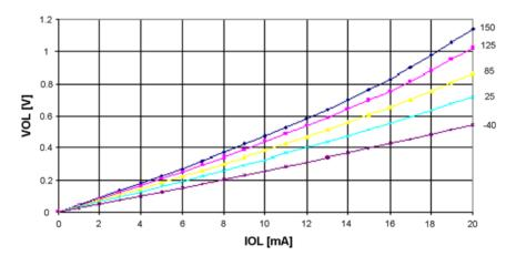
Figure 24-9. I/O Pin Output Voltage versus Sink Current ( $V_{CC} = 5V$ )
