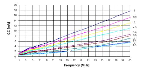
Figure 24-2. Active Supply Current versus Frequency (1 - 16MHz)
