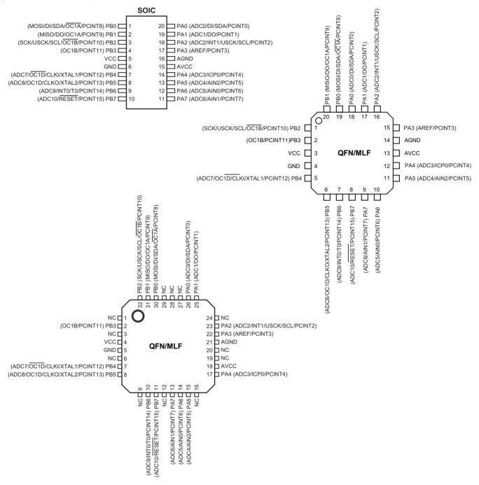
Note: The large center pad underneath the QFN/MLF package should be soldered to ground on the board to ensure good mechanical stability.
