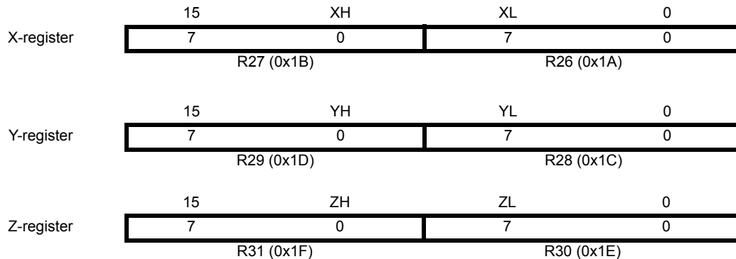
Figure 5-3. The X-, Y-, and Z-registers
