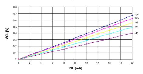
Figure 24-10. I/O Pin Output Voltage versus Source Current (V<sub>CC</sub> = 3V)
