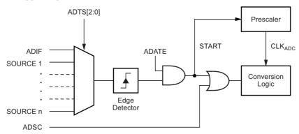
Using the ADC interrupt flag as a trigger source makes the ADC start a new conversion as soon as the ongoing conversion has finished. The ADC then operates in free running mode, constantly sampling and updating the ADC data register. The first conversion must be started by writing a logical one to the ADSC bit in ADCSRA. In this mode the ADC will perform successive conversions independently of whether the ADC interrupt flag, ADIF is cleared or not.
