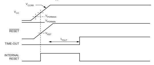
Figure 9-3. MCU Start-up, RESET Extended Externally
