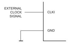
When this clock source is selected, start-up times are determined by the SUT fuses as shown in Table 7-3.
