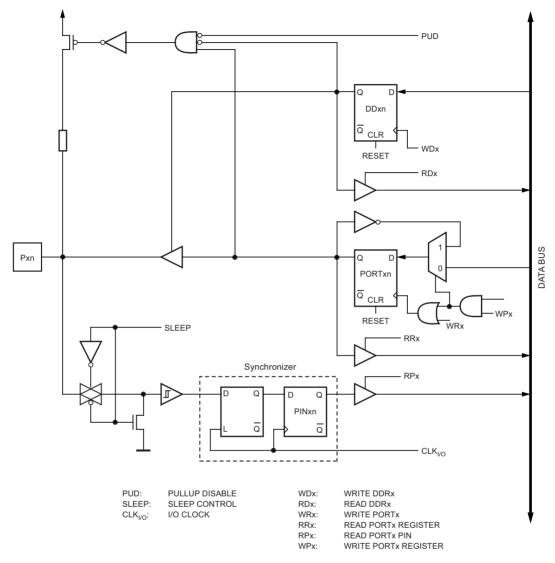
Note: WRx, WPx, WDx, RRx, RPx, and RDx are common to all pins within the same port. clk<sub>I/O</sub>, SLEEP, and PUD are common to all ports.
