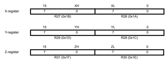
In the different addressing modes these address registers have functions as fixed displacement, automatic increment, and automatic decrement (see the instruction set reference for details).
