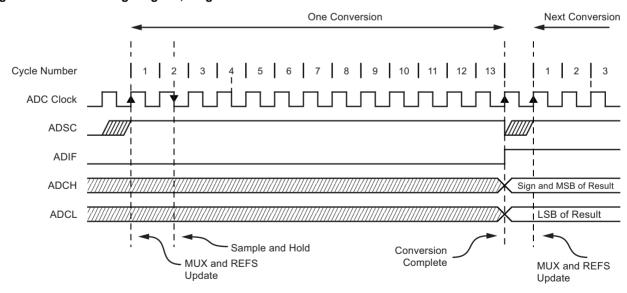
Figure 19-6. ADC Timing Diagram, Auto Triggered Conversion
