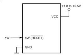
Figure 20-1 shows the schematic of a target MCU, with debugWIRE enabled, and the emulator connector. The system clock is not affected by debugWIRE and will always be the clock source selected by the CKSEL fuses.
