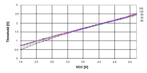
Figure 24-14. Reset Input Threshold Voltage versus V<sub>CC</sub> (V<sub>IH</sub>, Reset Read as '1')
