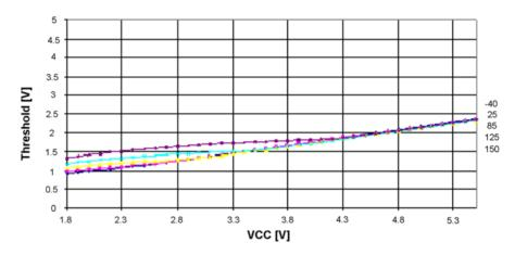
Figure 24-15. Reset Input Threshold Voltage versus  $V_{CC}$  ( $V_{IL}$ , Reset Read as '0')
