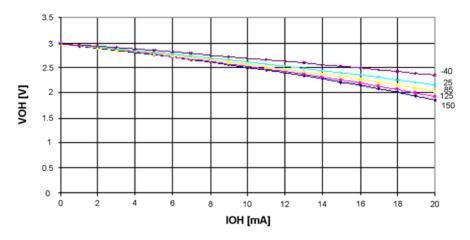
Figure 24-11. I/O Pin Output Voltage versus Source Current ( $V_{CC} = 5V$ )
