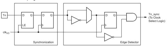
The synchronization and edge detector logic introduces a delay of 2.5 to 3.5 system clock cycles from an edge has been applied to the T0 pin to the counter is updated.
