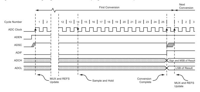
Figure 19-5. ADC Timing Diagram, Single Conversion
