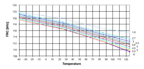
Figure 24-20. Calibrated 8.0MHz RC Oscillator Frequency versus Temperature
