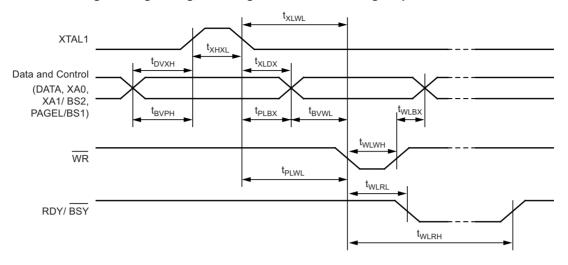
Figure 23-4. Parallel Programming Timing, Loading Sequence with Timing Requirements<sup>(1)</sup>
