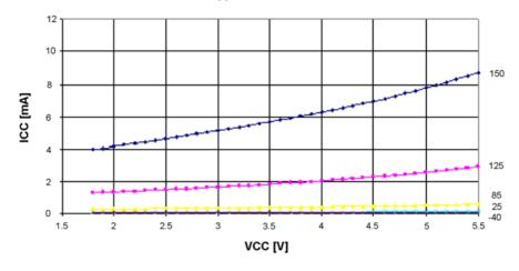
Figure 24-5. Power-down Supply Current versus V<sub>CC</sub> (Watchdog Timer Enabled)
