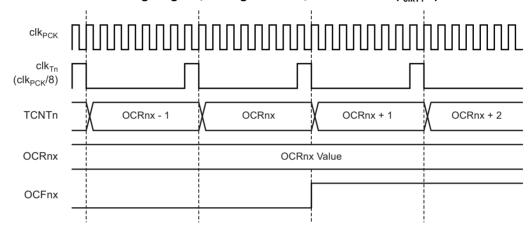
Figure 16-17. Timer/Counter Timing Diagram, with Prescaler (f<sub>clkT1</sub>/8)
