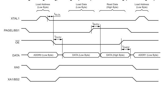
Note: 1. The timing requirements shown in Figure 23-3 on page 177 (i.e., t<sub>DVXH</sub>, t<sub>XHXL</sub>, and t<sub>XLDX</sub>) also apply to reading operation.
