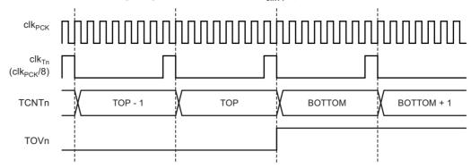
Figure 16-16. Timer/Counter Timing Diagram, Setting of OCF1x, with Prescaler (f<sub>clkT1</sub>/8)
