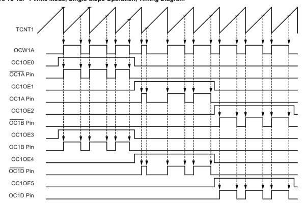
Figure 16-13. PWM6 Mode, Single-slope Operation, Timing Diagram
