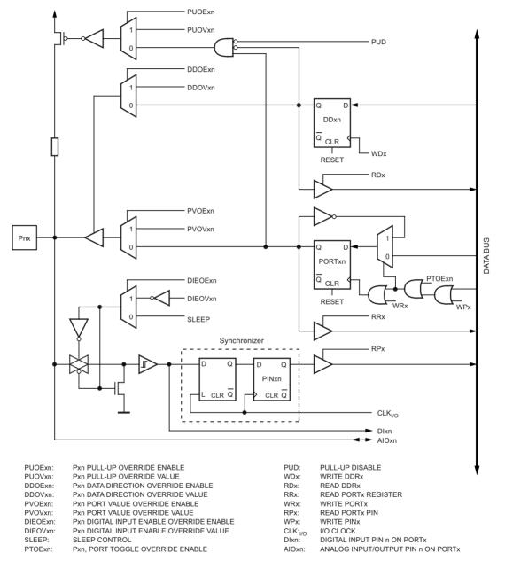
Note: WRx, WPx, WDx, RRx, RPx, and RDx are common to all pins within the same port. clk<sub>I/O</sub>, SLEEP, and PUD are common to all ports. All other signals are unique for each pin.
