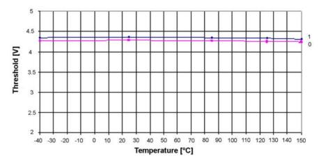
Figure 24-17. BOD Threshold versus Temperature (BOD Level is 2.7V)
