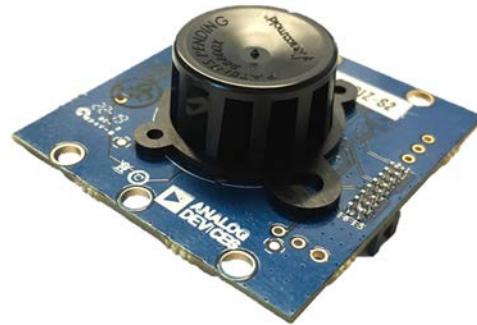
Figure 46. EVAL-CHAMBER Smoke Chamber
