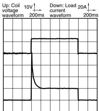
5-(3). Electrical life test (Motor load)
