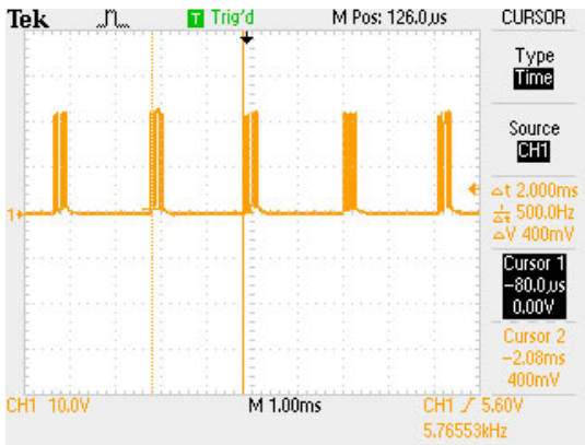
Figure 8. Cyclic data exchange every 2ms from the Santa Cruz to the IO-Link master.
