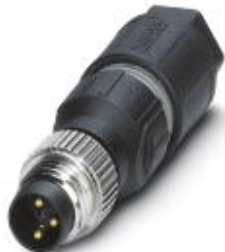
Sensor/actuator connector, male connector, straight, 3-pos., M8, metal knurl, maximum cable diameter of 5.0 mm
