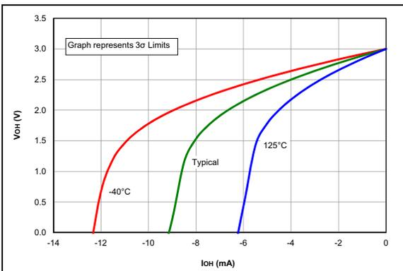
**FIGURE 27-39:**  $V_{OH}$  vs.  $I_{OH}$  Over Temperature,  $V_{DD} = 3.0V$ .
