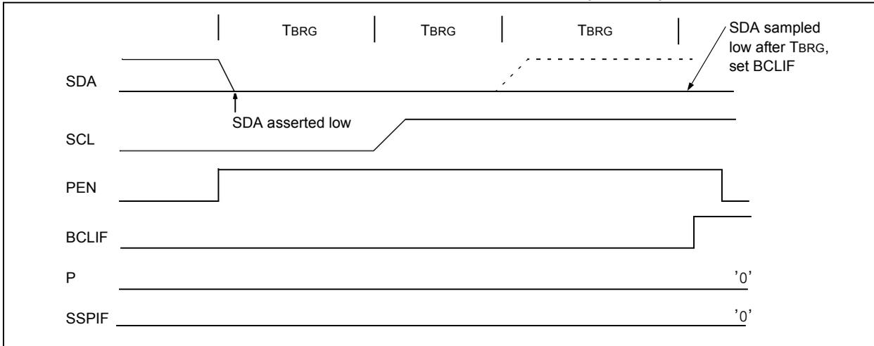
**FIGURE 23-39: BUS COLLISION DURING A STOP CONDITION (CASE 2)**
