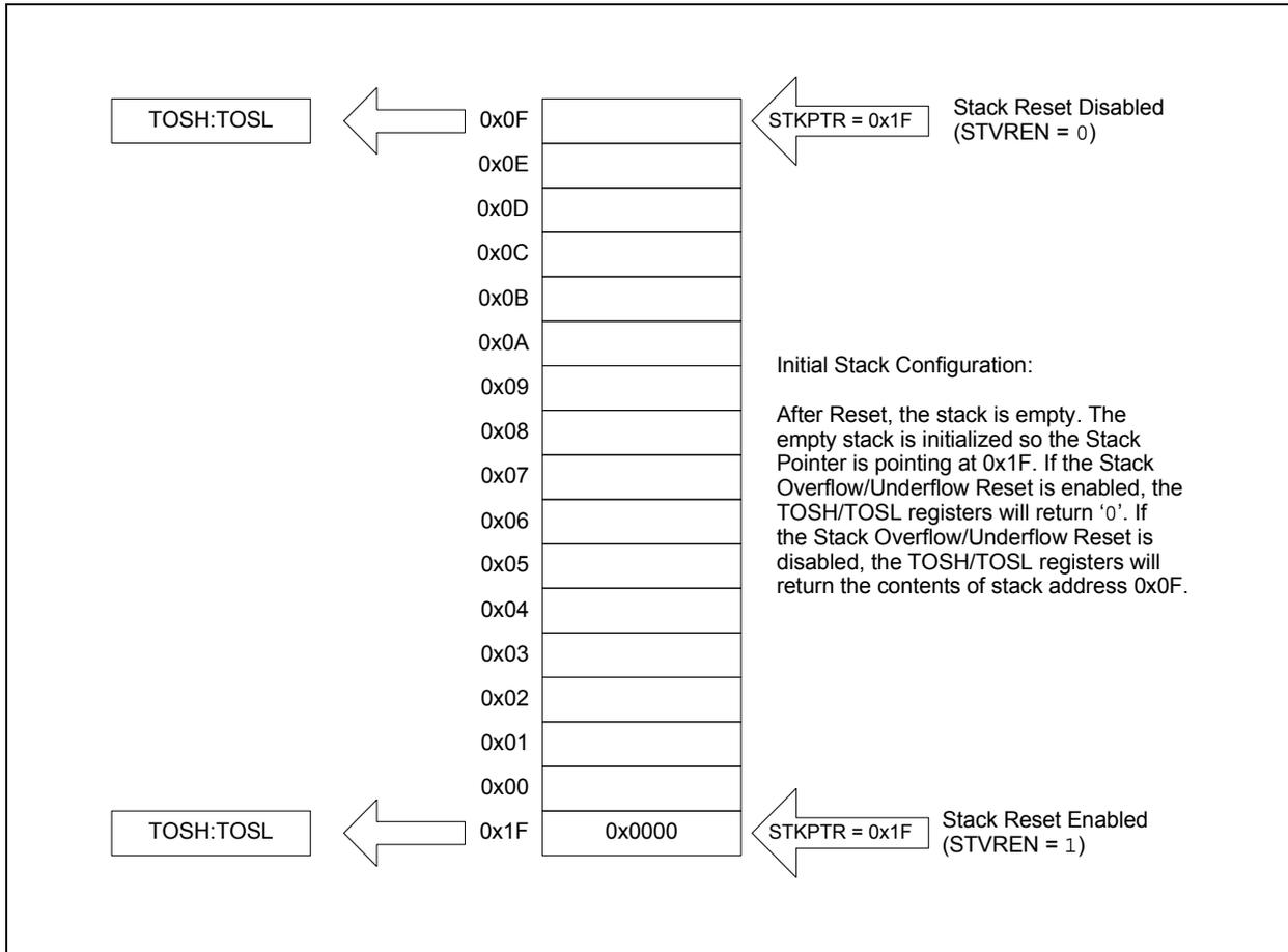
**FIGURE 3-5: ACCESSING THE STACK EXAMPLE 2**
