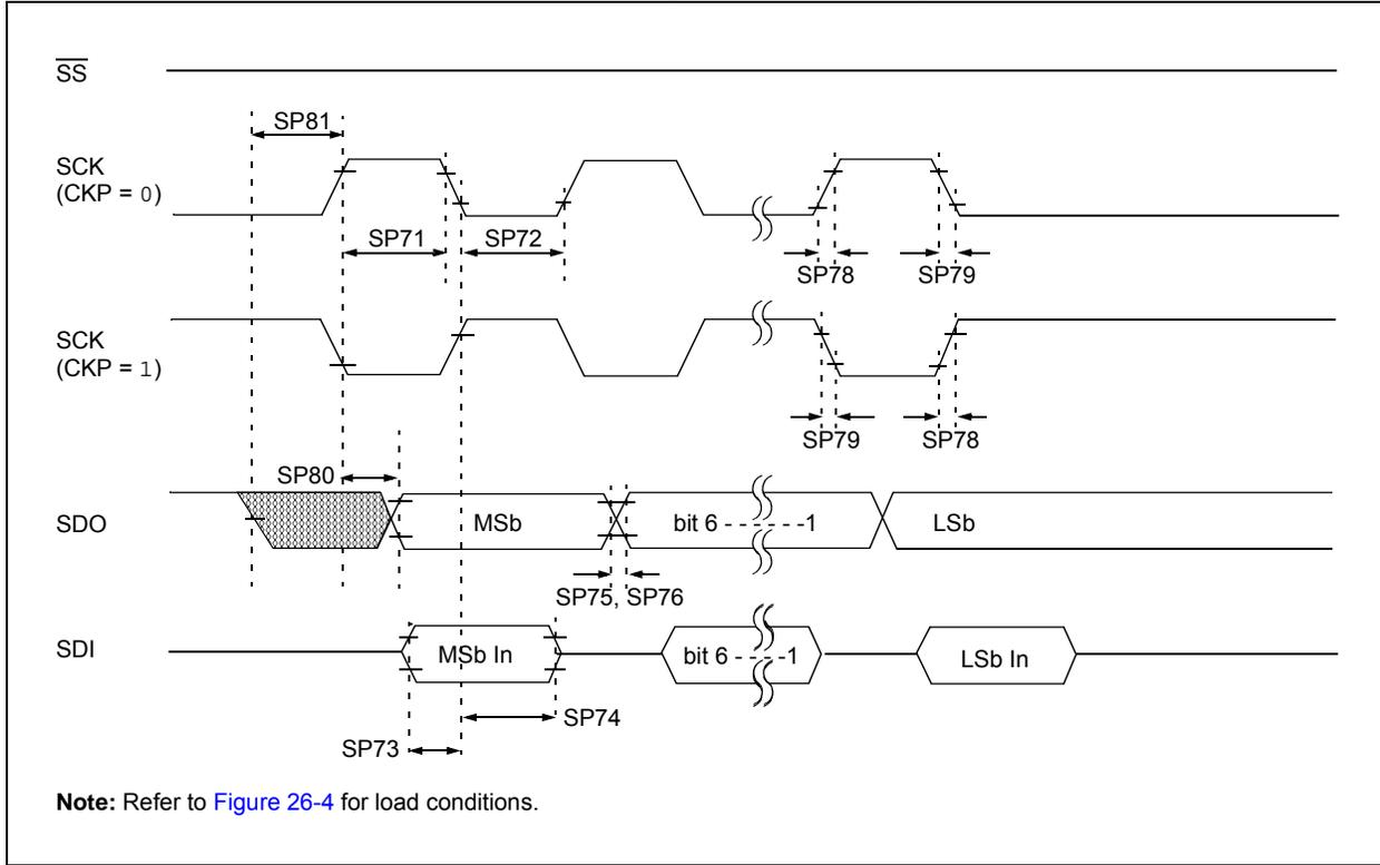
**FIGURE 26-15: SPI MASTER MODE TIMING (CKE = 1, SMP = 1)**
