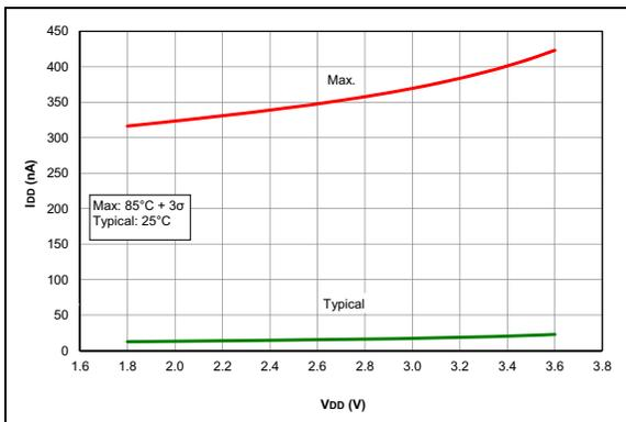
**FIGURE 27-21:**  $I_{PD}$  Base, Low-Power Sleep Mode, PIC16LF1703/7 Only.
