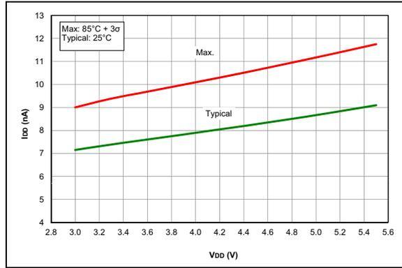
**FIGURE 27-28:**  $I_{PD}$ , Brown-Out Reset (BOR),  $BORV = 1$ , PIC16F1703/7 only.
