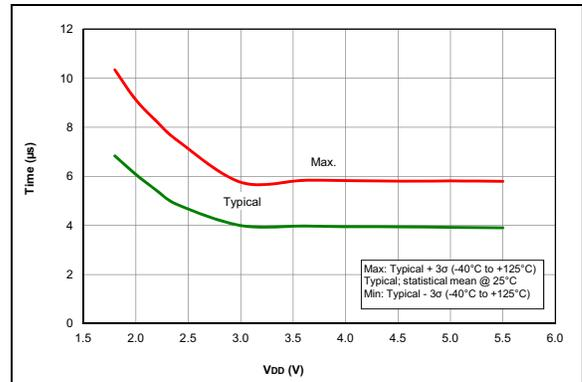
**FIGURE 27-60:** Wake From Sleep,  $V_{REGPM} = 0$ .
