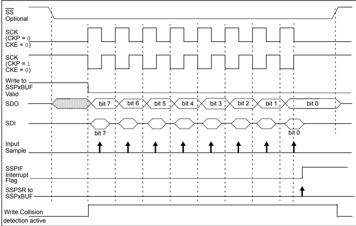
**FIGURE 23-10: SPI MODE WAVEFORM (SLAVE MODE WITH CKE = 1)**
