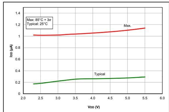
**FIGURE 27-36:**  $I_{DD}$ , ADC Non-Converting, PIC16F1703/7 only
