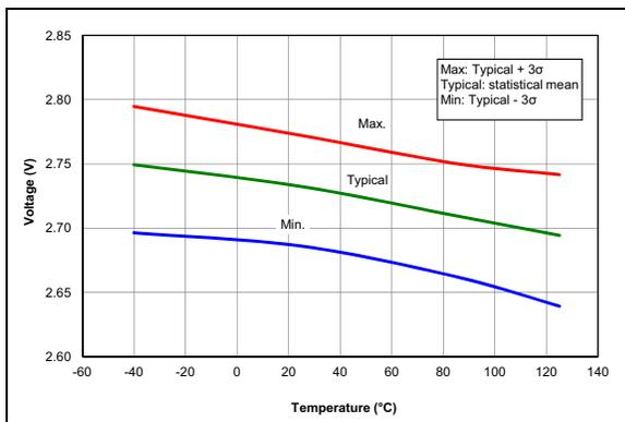
**FIGURE 27-51:** Brown-Out Reset Voltage, High Trip Point ( $BORV = 0$ ).
