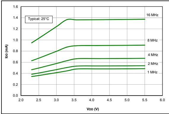
**FIGURE 27-19:**  $I_{DD}$  Typical, HFINTOSC Mode, PIC16F1703/7 Only.
