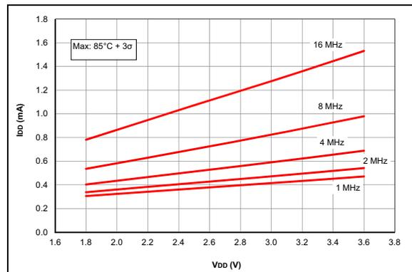
**FIGURE 27-18:**  $I_{DD}$  Maximum, HFINTOSC Mode, PIC16LF1703/7 Only.
