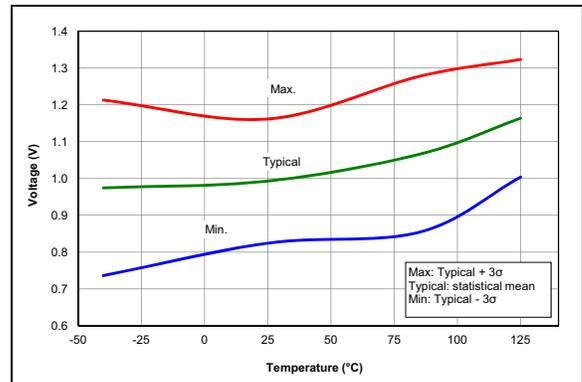
**FIGURE 27-59:** POR REARM Voltage, Normal-Power Mode, PIC16LF1703/7 Only.
