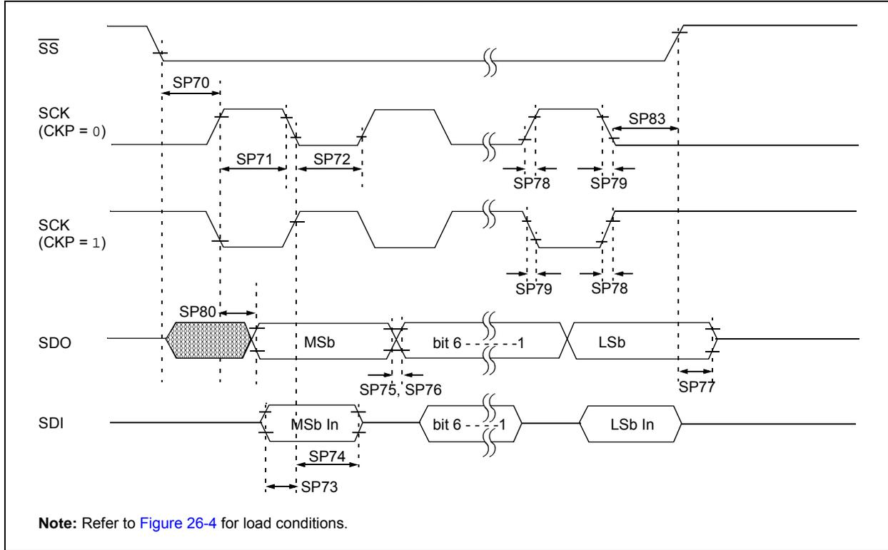
**FIGURE 26-17: SPI SLAVE MODE TIMING (CKE = 1)**
