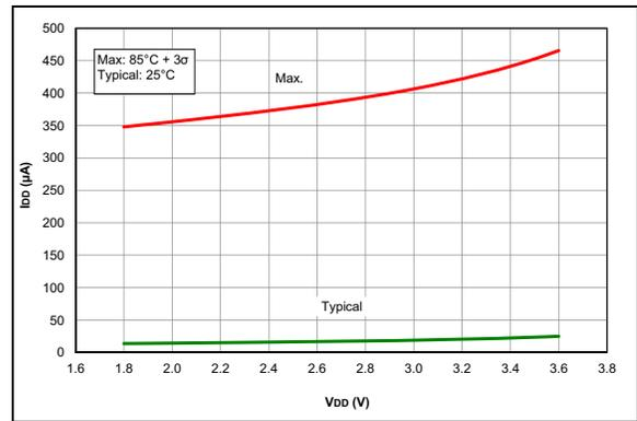
**FIGURE 27-35:**  $I_{DD}$ , ADC Non-Converting, PIC16LF1703/7 only
