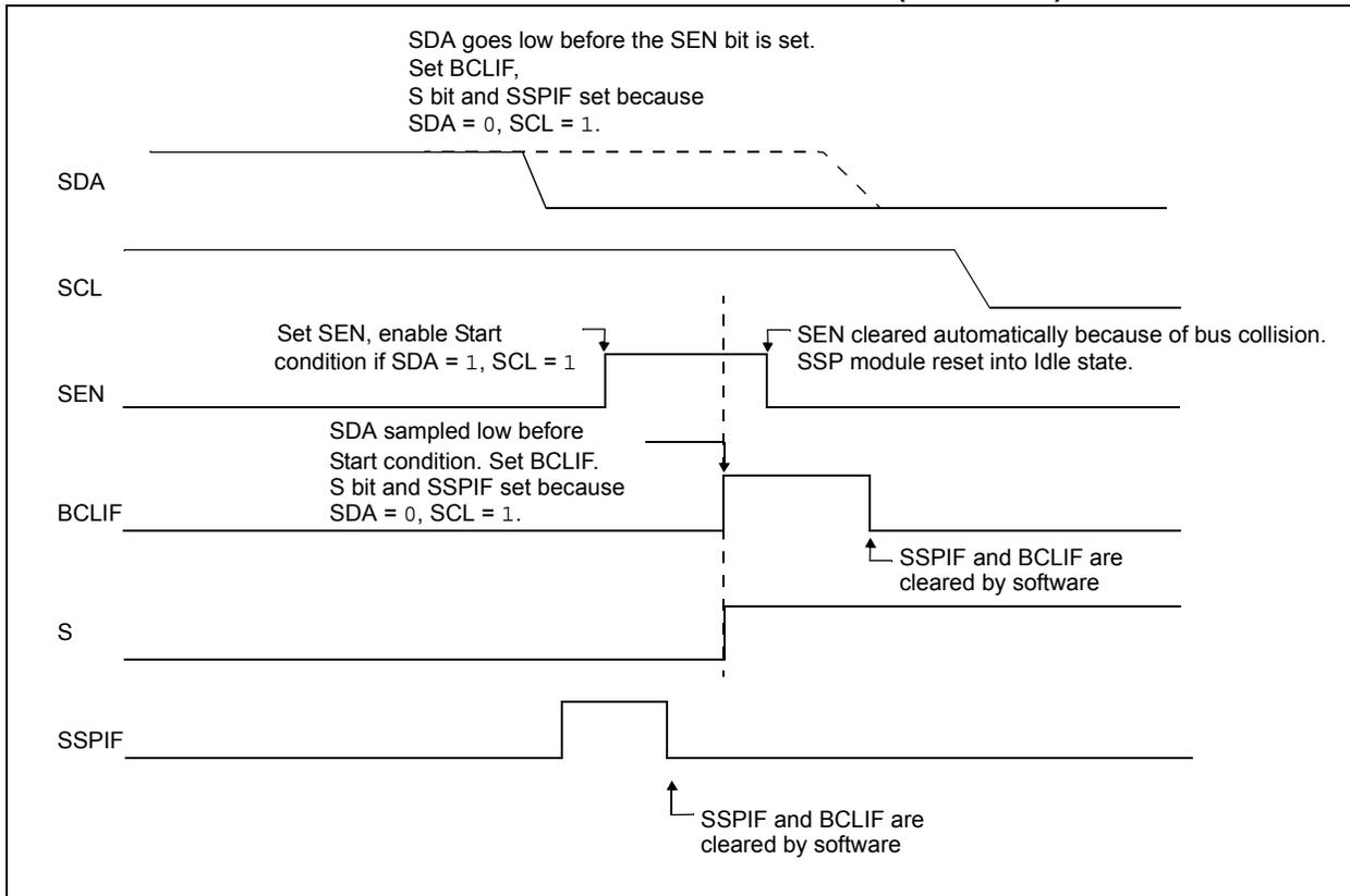
**FIGURE 23-34: BUS COLLISION DURING START CONDITION (SCL = 0)**
