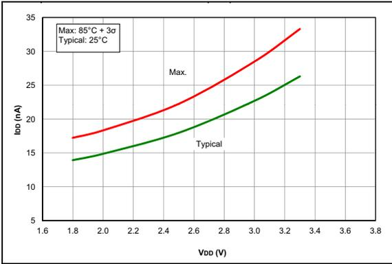
**FIGURE 27-25:**  $I_{PD}$ , Fixed Voltage Reference (FVR), PIC16LF1703/7 only.
