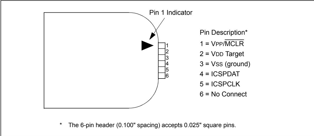
**FIGURE 24-3: TYPICAL CONNECTION FOR ICSP™ PROGRAMMING**
