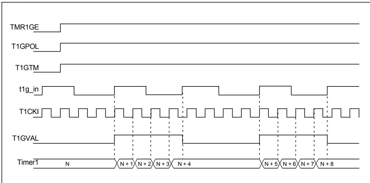
**FIGURE 20-5: TIMER1 GATE SINGLE-PULSE MODE**
