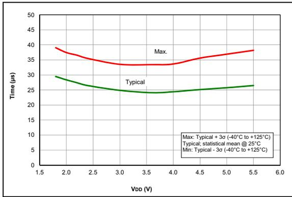
**FIGURE 27-61:** Wake From Sleep,  $V_{REGPM} = 1$ .
