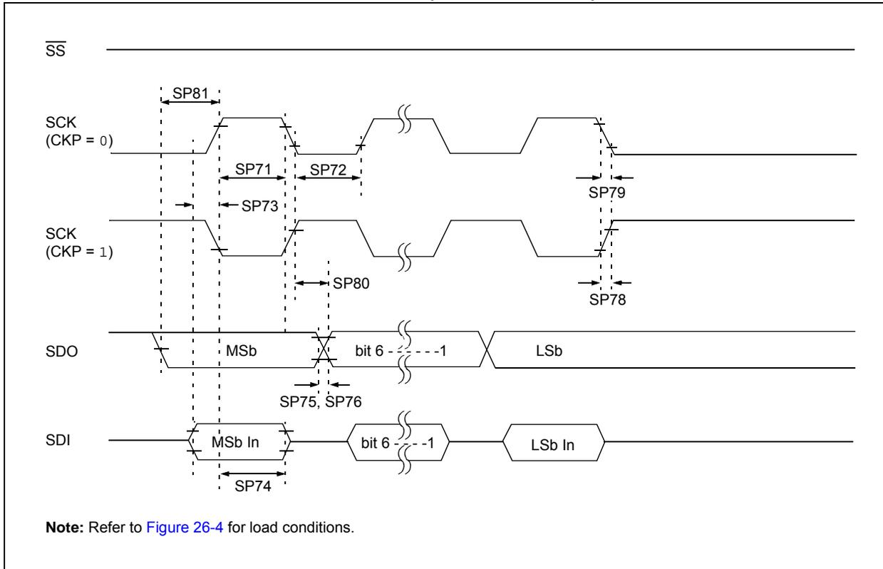
**FIGURE 26-16: SPI SLAVE MODE TIMING (CKE = 0)**
