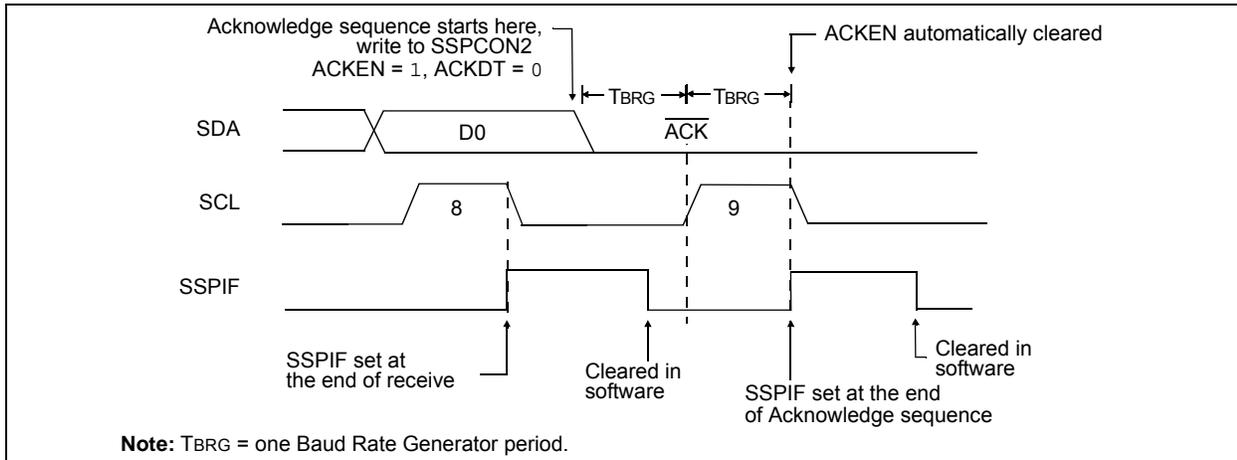
**FIGURE 23-31: STOP CONDITION RECEIVE OR TRANSMIT MODE**
