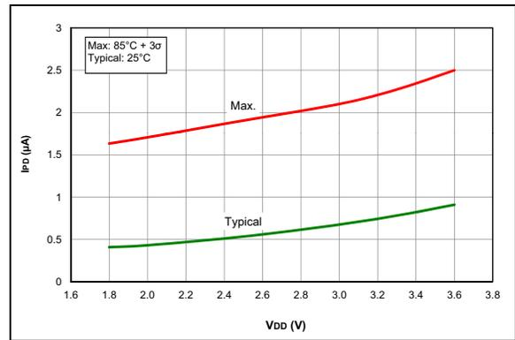
**FIGURE 27-23:**  $I_{PD}$ , Watchdog Timer (WDT), PIC16LF1703/7 only.
