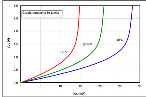
**FIGURE 27-40:**  $V_{OL}$  vs.  $I_{OL}$  Over Temperature,  $V_{DD} = 3.0V$ .
