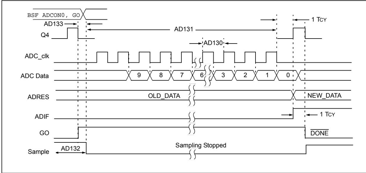
**FIGURE 26-13: ADC CONVERSION TIMING (ADC CLOCK FROM FRC)**
