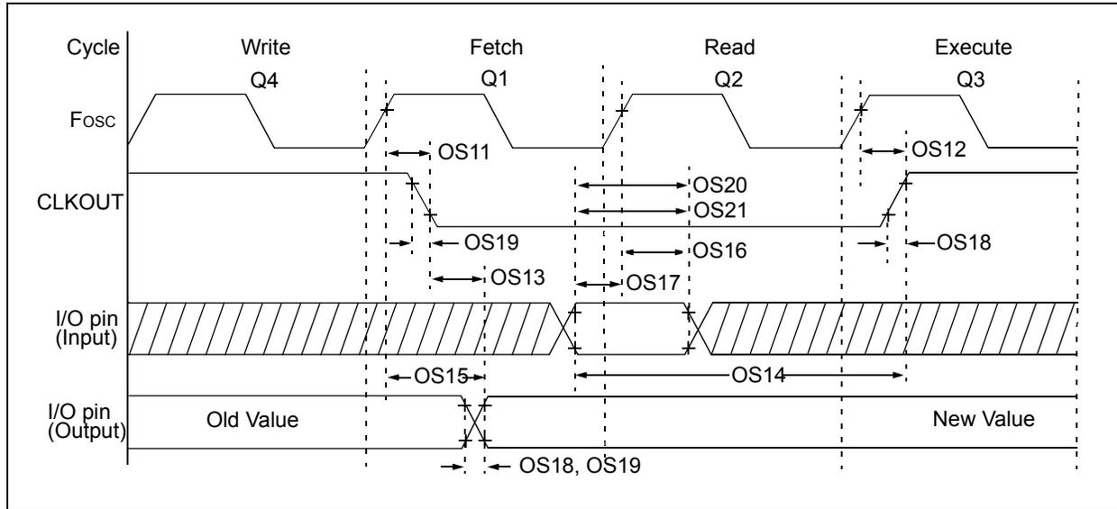
**TABLE 26-10: CLKOUT AND I/O TIMING PARAMETERS**
