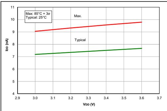
**FIGURE 27-27:**  $I_{PD}$ , Brown-Out Reset (BOR),  $BORV = 1$ , PIC16LF1703/7 only.
