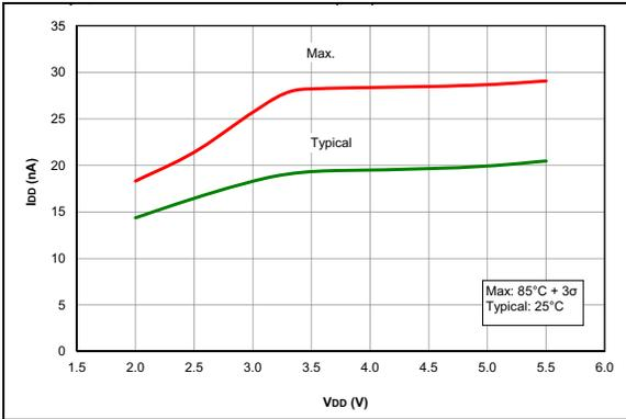
**FIGURE 27-26:**  $I_{PD}$ , Fixed Voltage Reference (FVR), PIC16F1703/7 only.
