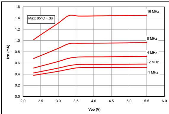
**FIGURE 27-20:**  $I_{DD}$  Maximum, HFINTOSC Mode, PIC16F1703/7 Only.
