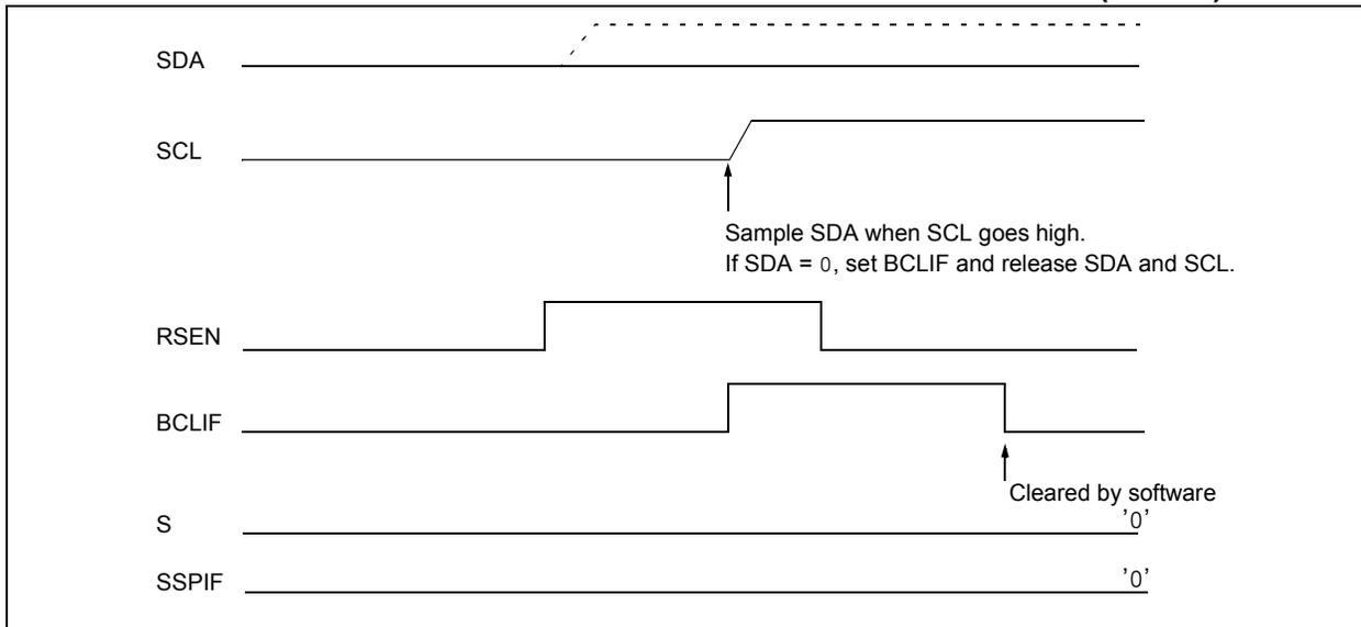
**FIGURE 23-37: BUS COLLISION DURING REPEATED START CONDITION (CASE 2)**
