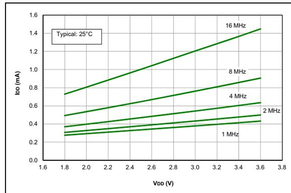
**FIGURE 27-17:**  $I_{DD}$  Typical, HFINTOSC Mode, PIC16LF1703/7 Only.
