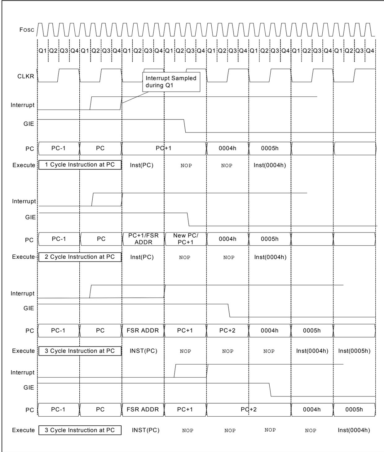
**FIGURE 7-3: INT PIN INTERRUPT TIMING**
