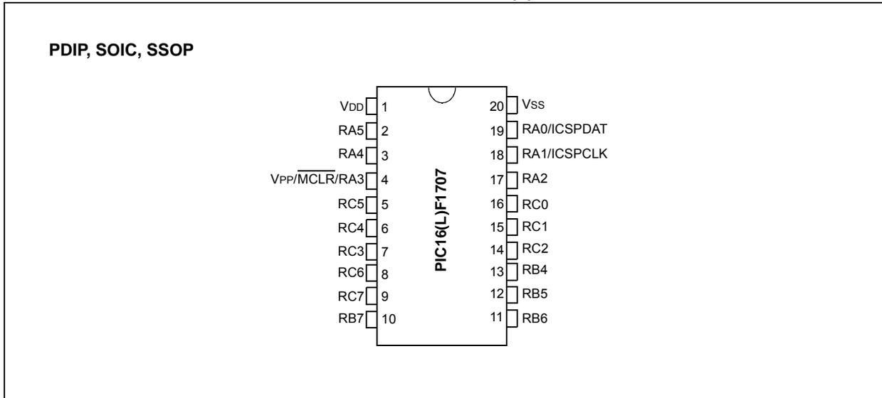
**FIGURE 4: 20-PIN PACKAGE DIAGRAM FOR PIC16(L)F1707**
