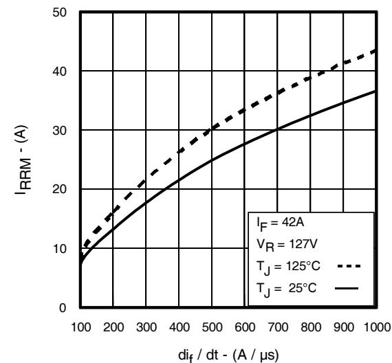
**Fig. 17 -** Typical Recovery Current vs.  $dI_f/dt$
