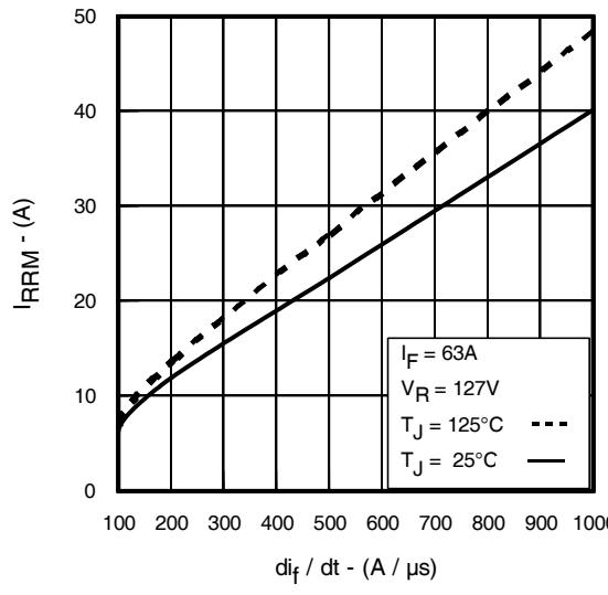
**Fig. 18 -** Typical Recovery Current vs.  $dI_f/dt$
