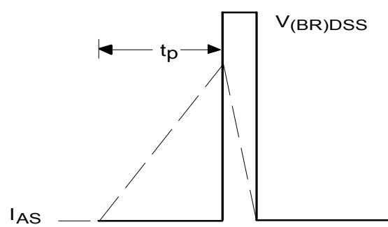
Fig 22b. Unclamped Inductive Waveforms
