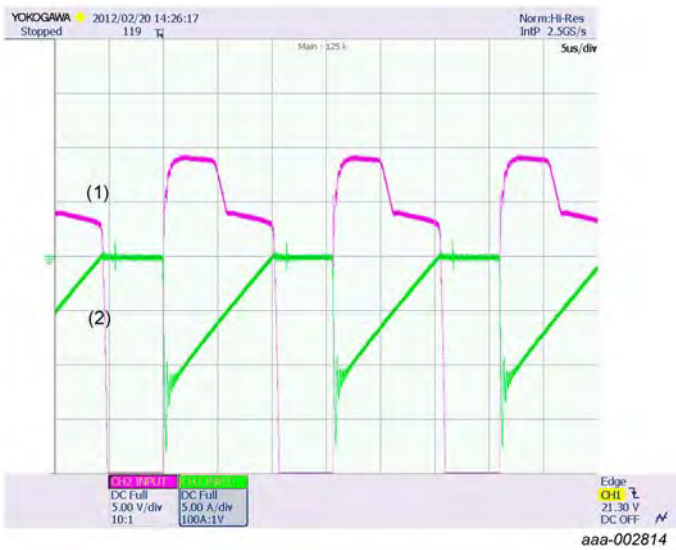
(1) Purple: gate drive current. (2) Green: secondary output current. b. 4 A load, SELREG pin connected to ground, regulation level –42 mV.
