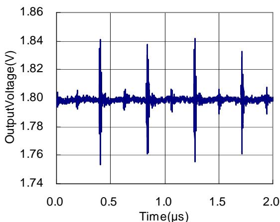
**RP501K181x(PWM/VFM mode change)** $V_{IN}=MODE=3.6V$ ,  $R_{OUT}=1\text{kohm}$
