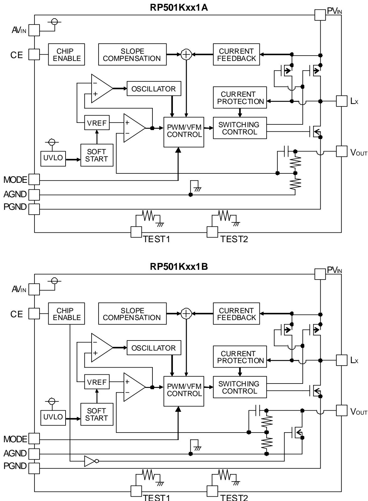
Mode="H": PWM/VFM alternative , Mode="L": PWM fix control
