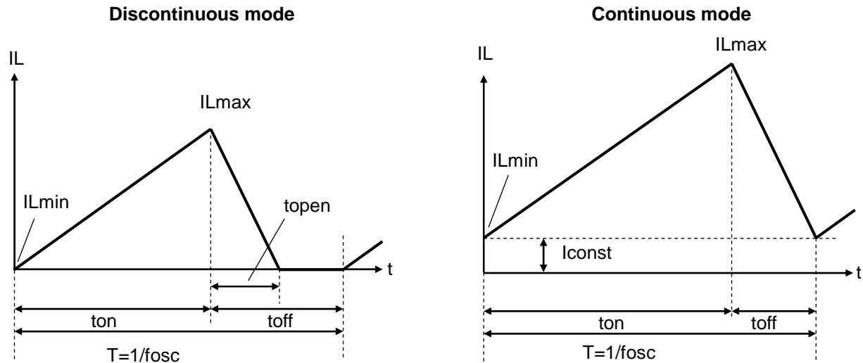
In the continuous mode, when Equation 1 is solved for  $t_{on}$  and assumed that the solution is  $t_{onc}$ ,
