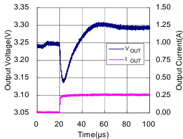
**RP501K331x** $V_{IN}=5.0V$ , MODE=5.0V,  $I_{OUT}=0.25A$  to  $0.001A$
