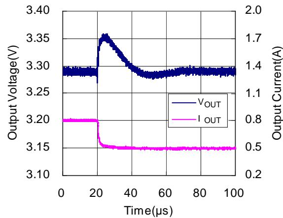
**RP501K331x** $V_{IN}=5.0V$ , MODE=5.0V,  $I_{OUT}=0.001A$  to  $0.25A$
