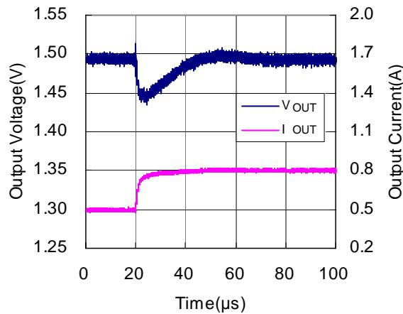
**RP501K151x** $V_{IN}=3.6V$ , MODE=0V,  $I_{OUT}=0.8A$  to  $0.5A$
