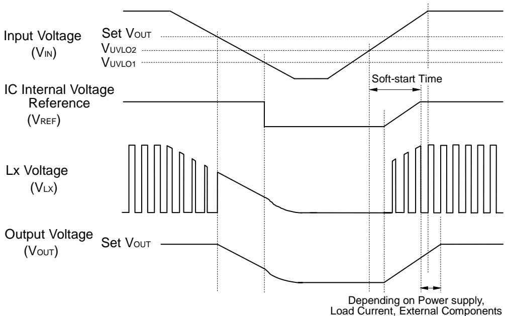
\*Actually, the waveform of  $V_{OUT}$  at UVLO working and releasing varies depending on the initial voltage of  $C_{OUT}$  and load current situation.
