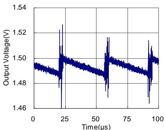
**RP501K181x(PWM fixed)** $V_{IN}=3.6V$ , MODE=0V,  $R_{OUT}=10\text{ohm}$
