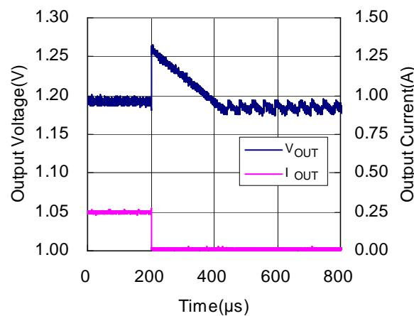
**RP501K151x** $V_{IN}=3.6V$ , MODE=0V,  $I_{OUT}=0.5A$  to  $0.8A$
