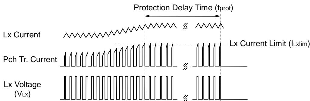
To release the condition of latch type protection, restart this IC by inputting "L" signal to CE pin, or restart this IC with power-on or make the supply voltage lower than UVLO detector threshold ( $V_{UVLO1}$ ) level.
