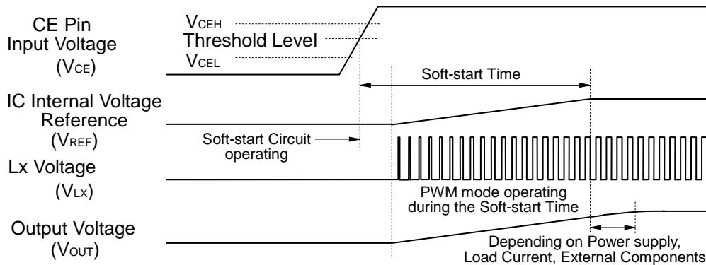
Soft-start time is the time interval from soft start circuit starting point to the reference voltage level reaching point up to this constant level.
