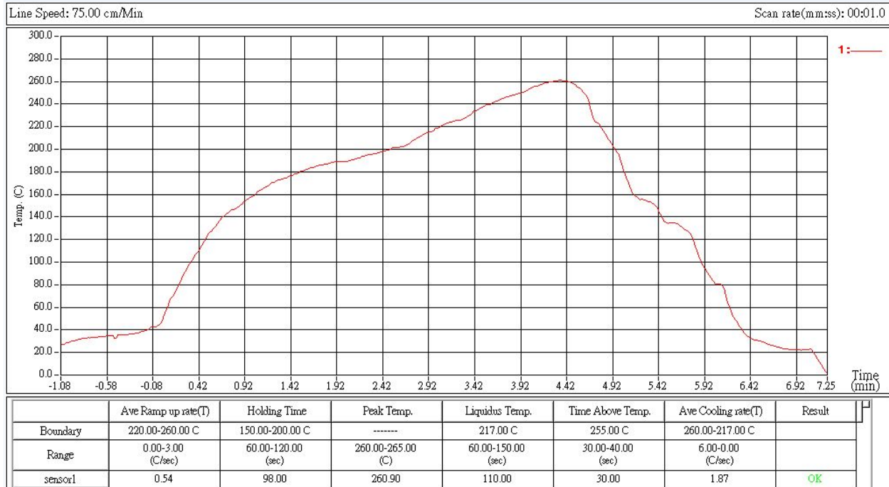
Figure 8.5 Solder Reflow Profile
