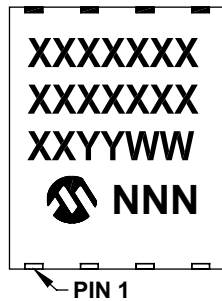
8-Lead DFN-S (6x5x0.9 mm)
