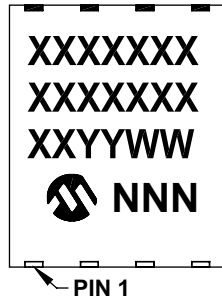
8-Lead DFN-S (6x5x0.9 mm)
