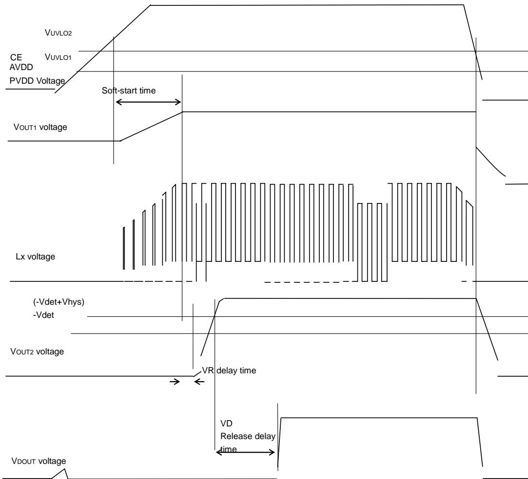
Timing chart of the power supply voltage change and DC/DC converter, VD, and VR can be explained as below:
