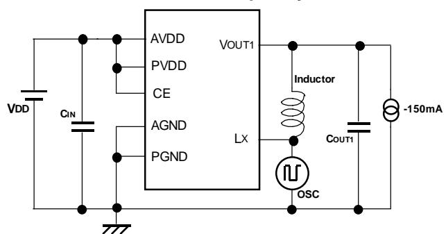
**UVLO Detect and Release Voltage Test Circuit**
