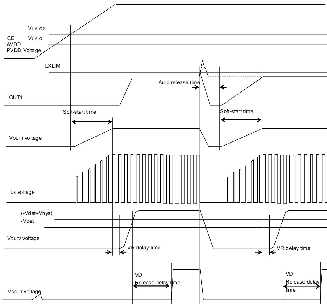
Timing chart of DC/DC converter output change by load, VD and VR can be explained as below:
