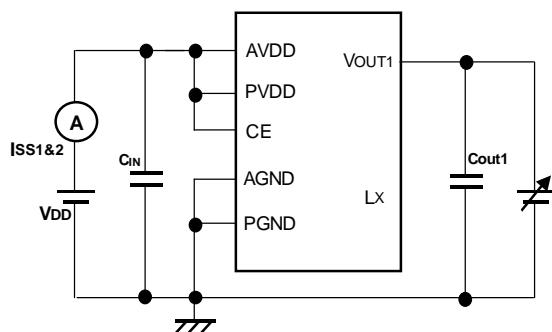
**DC/DC Output Voltage Test Circuit**
