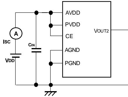
**VD Detect and Release Voltage Test Circuit**
