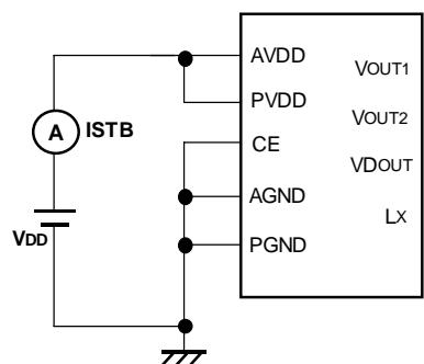
**Supply Current 1, 2 Test Circuit**
