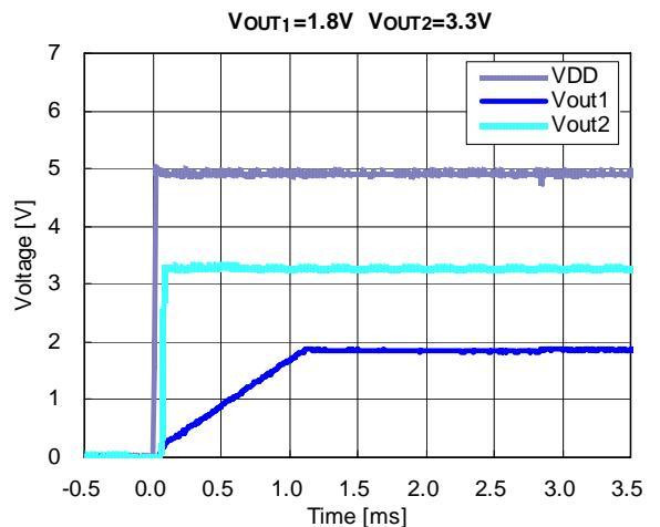
**22) VDOUT Release Delay Waveform (Version comparison)**
