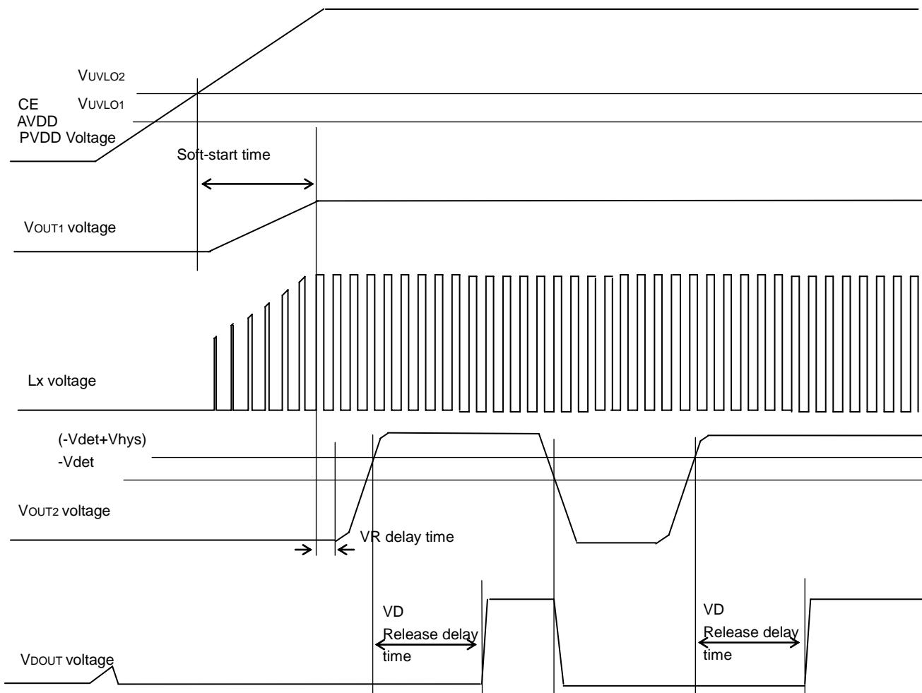
Timing chart of turning off by VR output voltage decreases, DC/DC converter, VD and VR can be explained as below:
