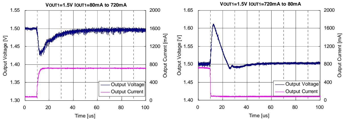
**24) VR Load transient response (DC/DC load current comparison)**
