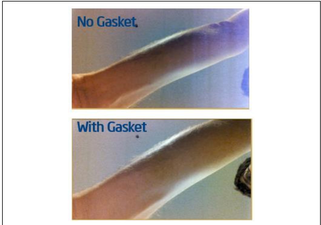
Figure 7-15. Example of Light Leakage Effects
