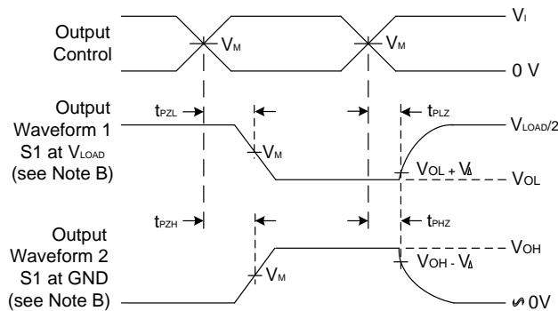
Figure 1 Load Circuit and Voltage Waveforms
