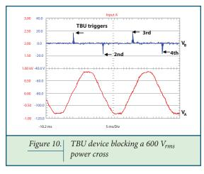
At the onset of the surge, the TBU device reacted to the increasing current and triggered to protect the load. The TBU device remained in the protected state throughout the remainder of the high voltage cycle. At each surge zero-crossing, the TBU device reset in a microsecond, and then retriggered to protect the load for each of the remaining cycles of the test. Once the fault was removed, the device reset to its normal, low impedance state.
