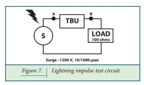
Figure 8 shows the input waveform on the lower trace in red (voltage on the TBU device input,  $V_A$ ) and the voltage at the TBU device output on the upper trace in blue ( $V_B$ ). The TBU device current limited to ~280 ma (i.e. 28 V across the 100  $\Omega$  resistor) and then disconnected the load throughout the remainder of the surge. The peak voltage across the TBU device was ~1200 V, just after it triggered to protect the load. The device automatically reset after the surge ended.
