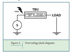
A lightning or power cross event at time 1 (see figure 6), raises the voltage and current until the current limiting portion of the circuit limits current to the level of  $I_{out}$  time 2 (~10 nanoseconds). At this point, the voltage disconnect portion of the circuit operates and by time 3 (~ 1 microsecond), the load is disconnected from the surge. During the remainder of the surge (time 4), the TBU device remains in the protected state of very low current and voltage at the load.
