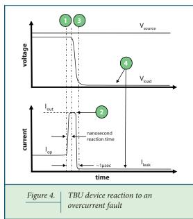
High-Speed Electronic Current Limiter
