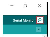
Then, when the serial monitor window opens, be sure the drop-down menus in the bottom right corner are configured to a baud rate of 9600 and the line terminator is set to Both NL & CR.
