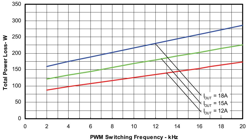
Figure 5. Total Power Losses vs. PWM Switching Frequency
