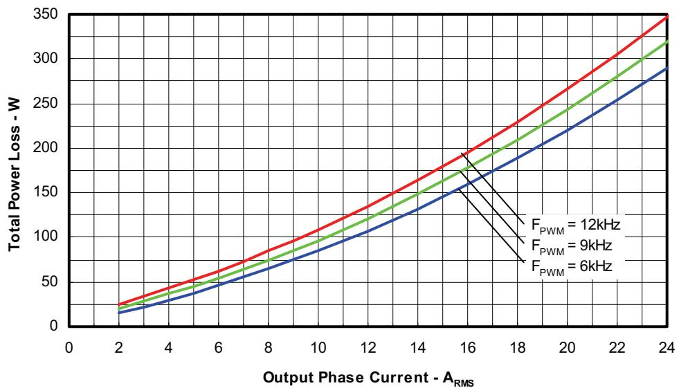
Figure 6. Total Power Losses vs. Output Phase Current
