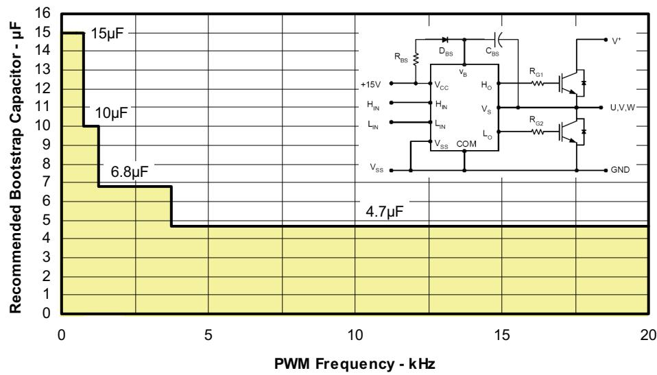
Figure 10. Recommended Bootstrap Capacitor Value vs. Switching Frequency
