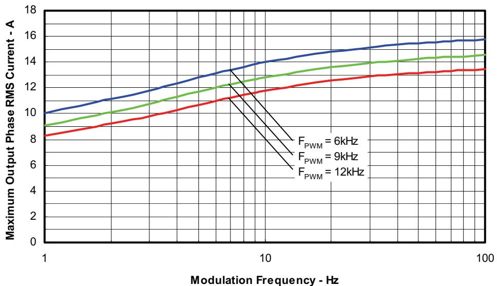
Figure 4. Maximum Sinusoidal Phase Current vs. Modulation Frequency
