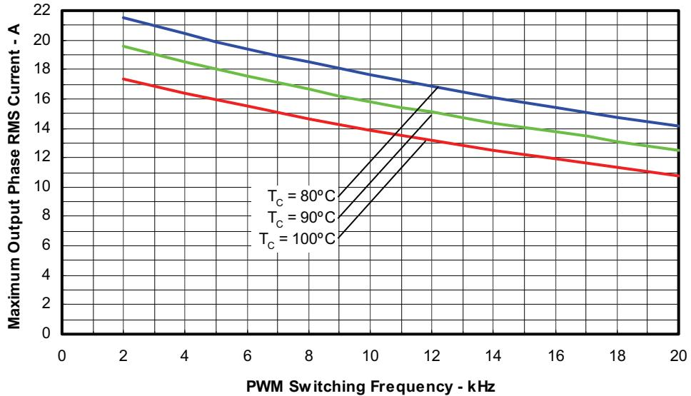
Figure 3. Maximum Sinusoidal Phase Current vs. PWM Switching Frequency
