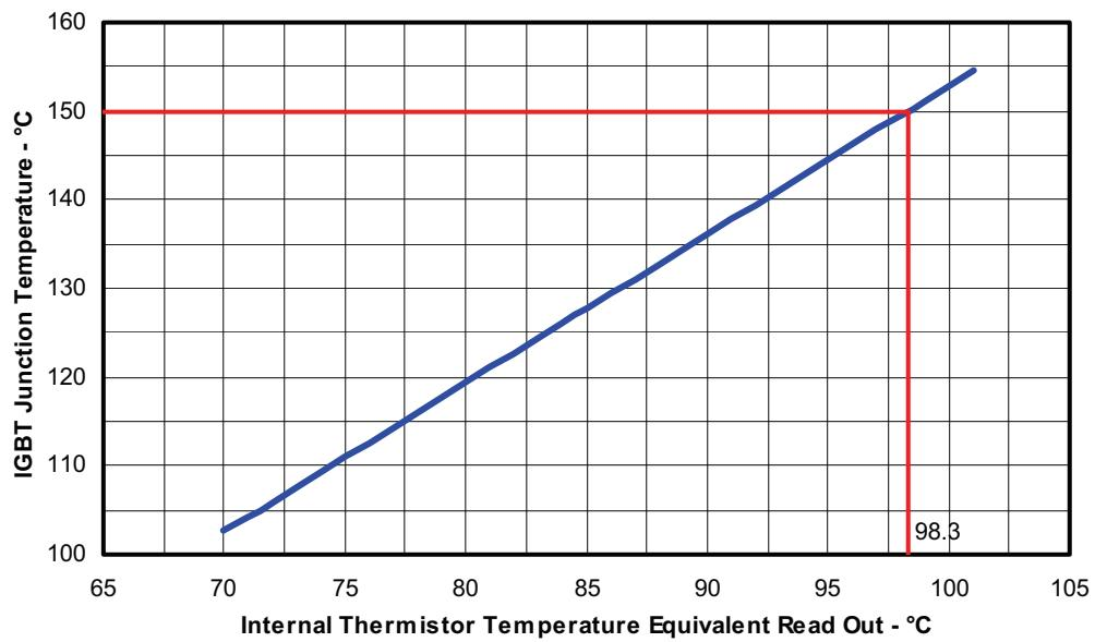
Figure 8. Estimated Maximum MOSFET Junction Temperature vs. Thermistor Temperature
