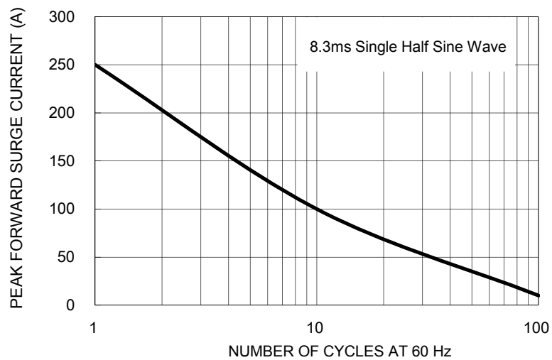
FIG. 9- MAXIMUM NON-REPETITIVE PEAK FORWARD SURGE CURRENT
