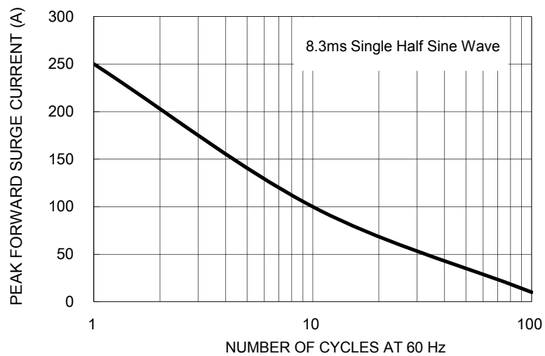
FIG. 9- MAXIMUM NON-REPETITIVE PEAK FORWARD SURGE CURRENT
