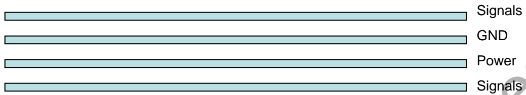
Figure 29: Typical 4-layer PCB construction
