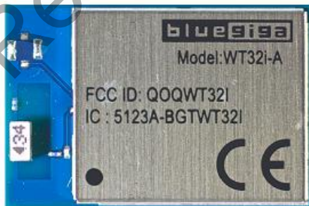
Figure 1: WT32i Bluetooth Audio Module
