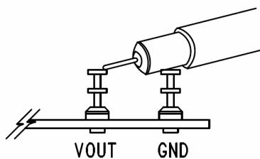
Figure 2. Measuring Output or Input Voltage Ripple
