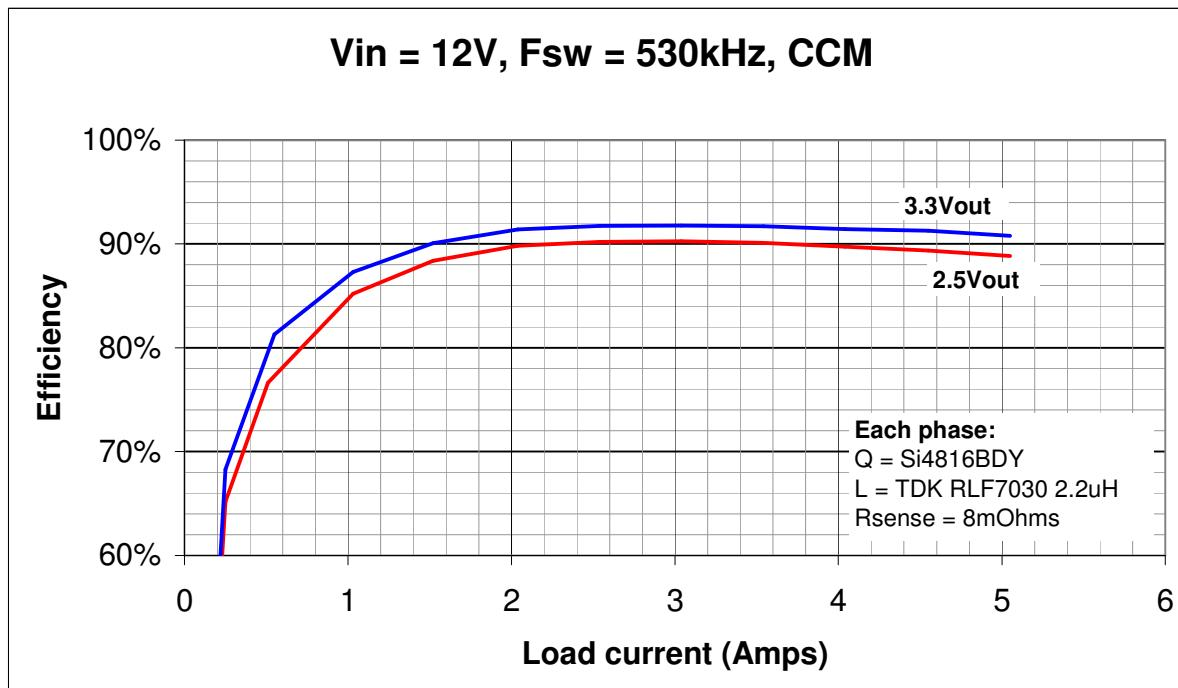
Figure 3. Typical Efficiency vs Load Current
