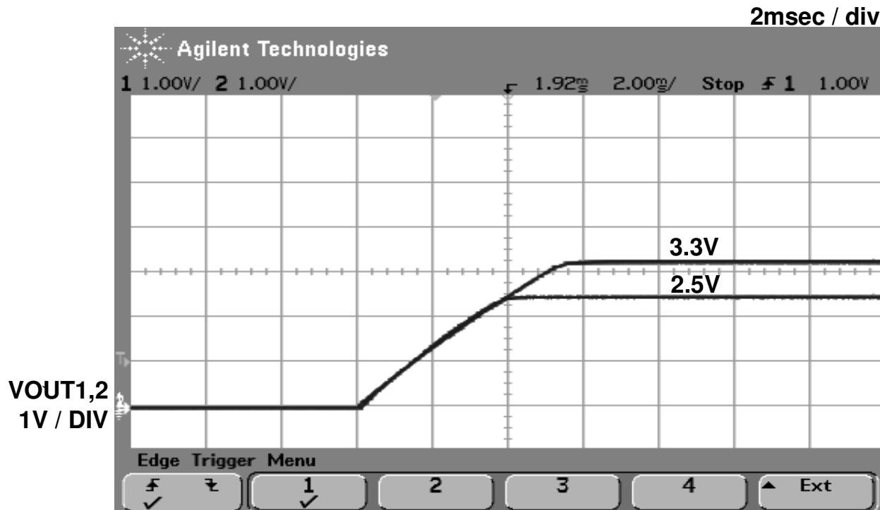
Figure 4. Coincident Rail Tracking During Startup (original board).
