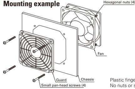
Plastic finger guards are placed on both the intake and exhaust sides of the fan.
