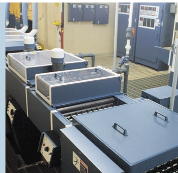
Photo-chemical machining produces extremely intricate and complex parts to precise specifications and provides a cost-effective alternative to tooling.
