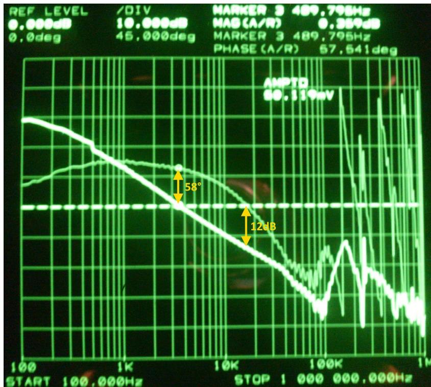
Figure 6. Gain and Phase Margin of the Flyback DC/DC Converter (Conditions:
