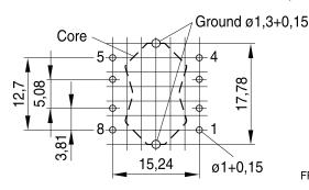
Hole arrangement View in mounting direction
