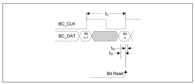
FIGURE 30-13: BC-LINK WRITE TIMING
