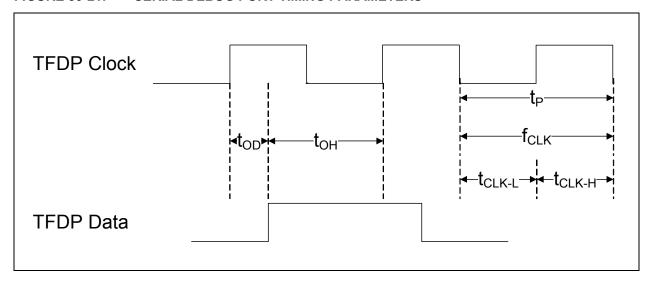
TABLE 30-16: SERIAL DEBUG PORT INTERFACE TIMING PARAMETERS
