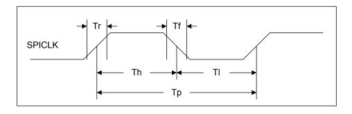
**TABLE 30-14: SPI CLOCK TIMING PARAMETERS**
