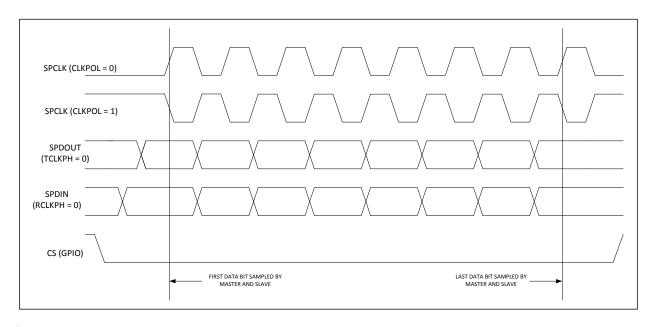
In this mode, data is available immediately when a device is selected and is sampled on the first and following odd SPCLK edges by the master and slave.
