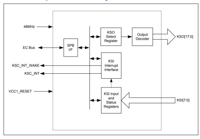
During scanning the firmware sequentially drives low one of the rows (KSO[17:0]) and then reads the column data line (KSI[7:0]). A key press is detected as a zero in the corresponding position in the matrix. Keys that are pressed are debounced by firmware. Once confirmed, the corresponding keycode is loaded into host data read buffer in the 8042 Host Interface module. Firmware may need to buffer keycodes in memory in case this interface is stalled or the host requests a Resend.
