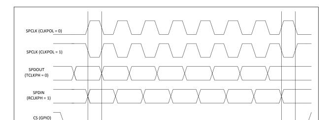
FIGURE 30-19: SPI INTERFACE TIMING, FULL DUPLEX MODE (TCLKPH = 0, RCLKPH = 1)
