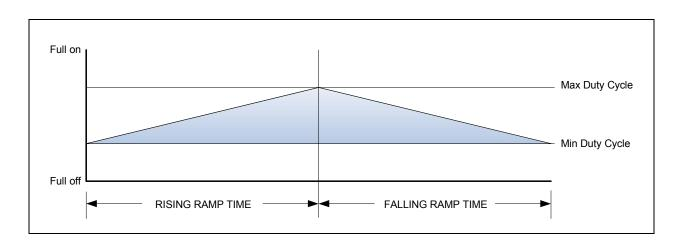
The breathing range of and LED can range between full on and full off, or in a range that falls within the full-on/full-off range, as shown in this figure. The ramp time can be different in different applications. For example, if the ramp time was 1 second, the LED would appear to breathe quickly. A time of 2 seconds would make the LED appear to breathe more leisurely.
