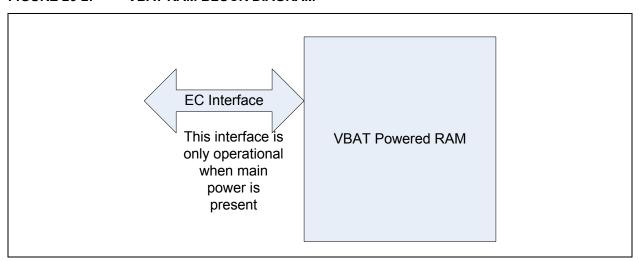
The VBAT Powered RAM provides a 64 Byte Random Accessed Memory that is operational while VCC1 is powered, and will retain its values powered by VBAT while VCC1 is unpowered. The RAM is organized as a 16 words x 32-bit wide for a total of 64 bytes.
