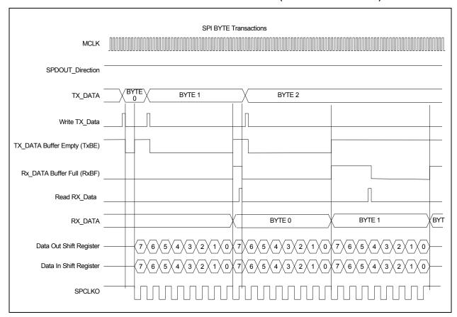
FIGURE 20-3: MULTI-BYTE SPI TX/RX TRANSACTIONS (FULL DUPLEX MODE)
