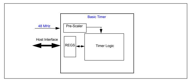
This timer block offers a simple mechanism for firmware to maintain a time base in the design. The timer may be enabled to execute the following features:
