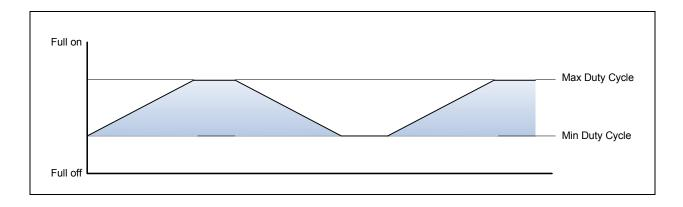
The clipping periods at the two extremes can be adjusted independently, so that for example an LED can appear to breathe (with a short delay at maximum brightness) followed by a longer "resting" period (with a long delay at minimum brightness).
