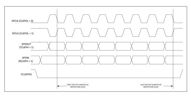
In this mode, the master and slave require an initial SPCLK edge before data is available. Data is sampled on the second and following even SPCLK edges by the master and slave.
