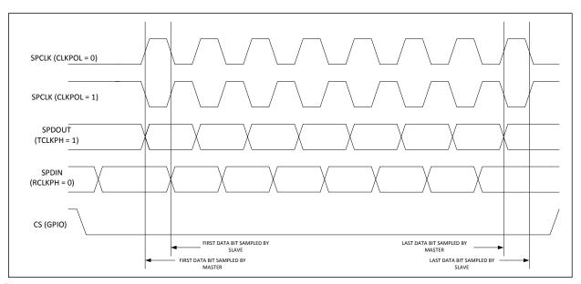
In this mode, the master requires an initial SPCLK edge before data is available. The data from slave is available immediately when the slave device is selected. The data is sampled on the first and following odd edges by the master. The data is sampled on the second and following even SPCLK edges by the slave.
