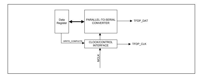
The firmware executing on the embedded controller writes to the Debug Data Register to initiate a transfer cycle. At first, data from the Debug Data Register is shifted into the LSB. Afterwards, it is transmitted at the rate of one byte per transfer cycle.
