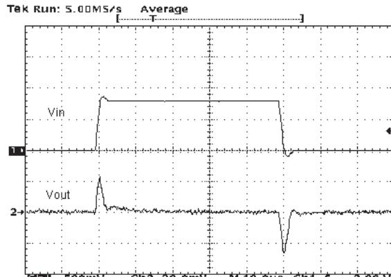
$V_O = 2.5$  V,  $I_O = 50$  mA, no  $C_l$ ,  $C_O = 4.7$   $\mu$ F,  $t_r = t_f = 1$   $\mu$ s
