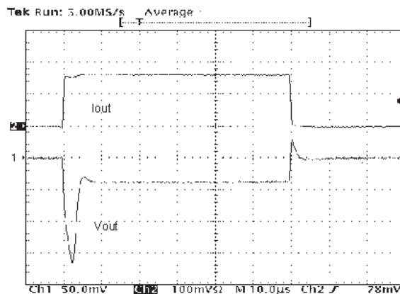
$V_O = 2.5$  V,  $I_O = 0$  to 50 mA, no  $C_l$ ,  $C_O = 4.7$   $\mu$ F,  $t_r = t_f = 500$  ns
