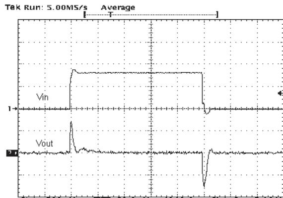
$V_O = 2.5$  V,  $I_O = 50$  mA, no  $C_l$ ,  $C_O = 4.7$   $\mu$ F,  $t_r = t_f = 500$  ns
