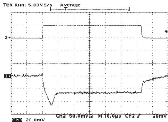
$V_O = 2.5$  V,  $I_O = 0$  to 50 mA, no  $C_l$ ,  $C_O = 10$   $\mu$ F,  $t_r = t_f = 500$  ns
