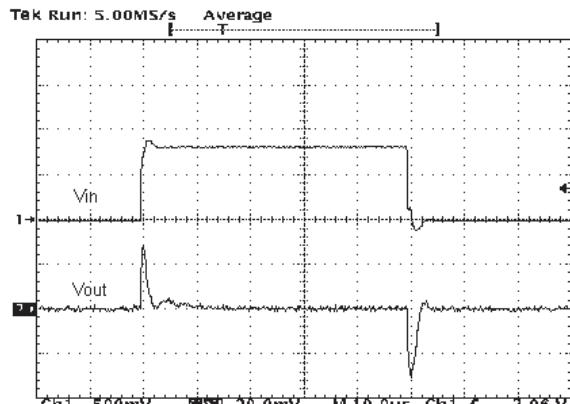
$V_O = 2.5$  V,  $I_O = 50$  mA, no  $C_I$ ,  $C_O = 4.7$   $\mu$ F,  $t_r = t_f = 500$  ns
