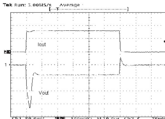
$V_O = 2.5$  V,  $I_O = 0$  to 50 mA, no  $C_I$ ,  $C_O = 4.7$   $\mu$ F,  $t_r = t_f = 500$  ns
