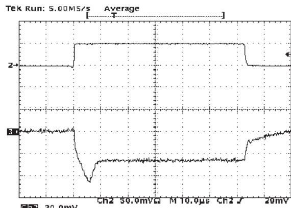
$V_O = 2.5$  V,  $I_O = 0$  to 50 mA, no  $C_I$ ,  $C_O = 10$   $\mu$ F,  $t_r = t_f = 500$  ns
