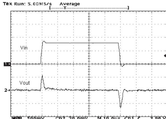
$V_O = 2.5$  V,  $I_O = 50$  mA, no  $C_I$ ,  $C_O = 4.7$   $\mu$ F,  $t_r = t_f = 1$   $\mu$ s
