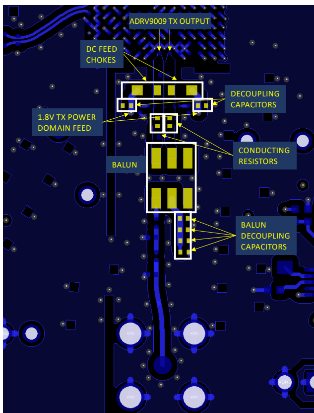
Figure 443. Transmitter DC Chokes and Balun Feed Supply
