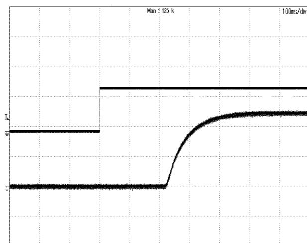
**Figure 8:** Vout start up with Enable on at 72Vin, 12.5A Iout,
