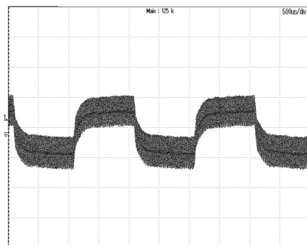
**Figure 7:** Dynamic response to load step 6.25A~9.375A with 0.1A/uS slew rate at 72Vin
