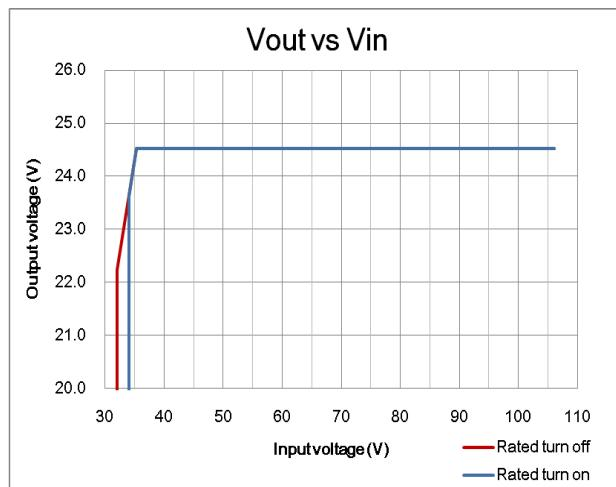
**Figure 2:** Vout vs. Vin @ Full load
