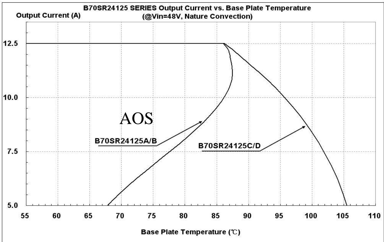
Figure 18: Output Power vs. base plate temperature @Vin=48V
