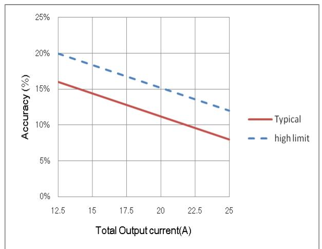
**Figure 6:** Current share accuracy vs. Total output current
