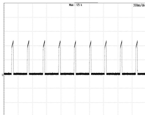
**Figure 11:** Output short current @ Vin=72V
