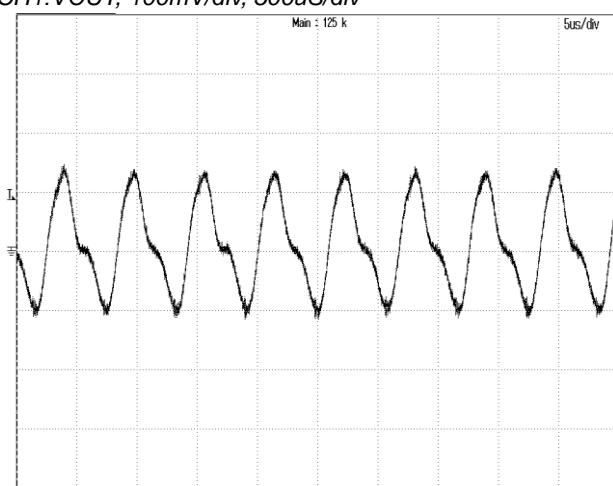
**Figure 9:** Output ripple & noise at 72Vin, 24A Iout
