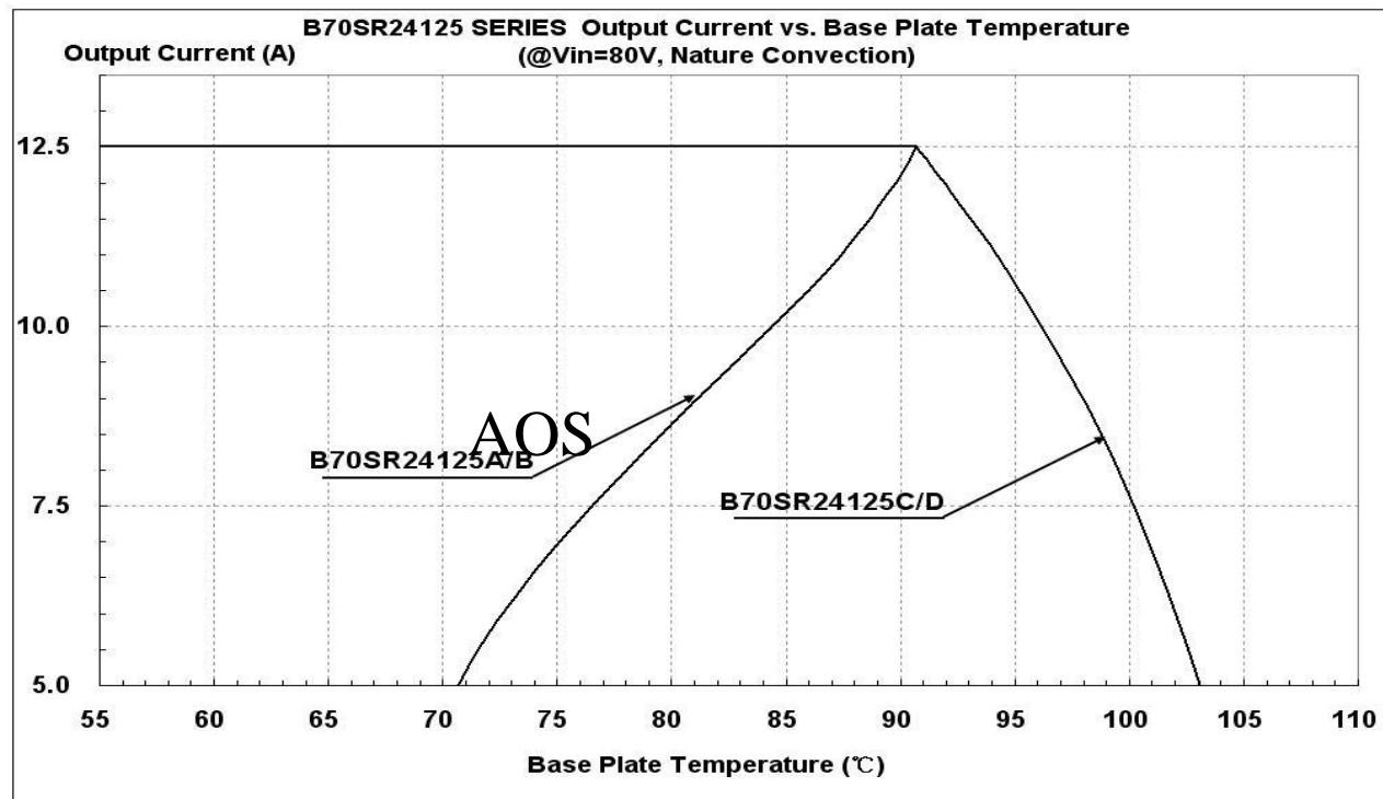
Figure 20: Output Power vs. base plate temperature @ $V_{in}=80V$
