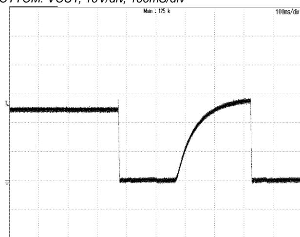
**Figure 10:** Output over voltage protection at 72Vin, 24A Iout
