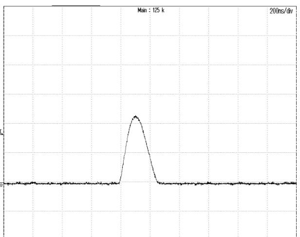
**Figure 12:** Inrush current @ Vin=72V
