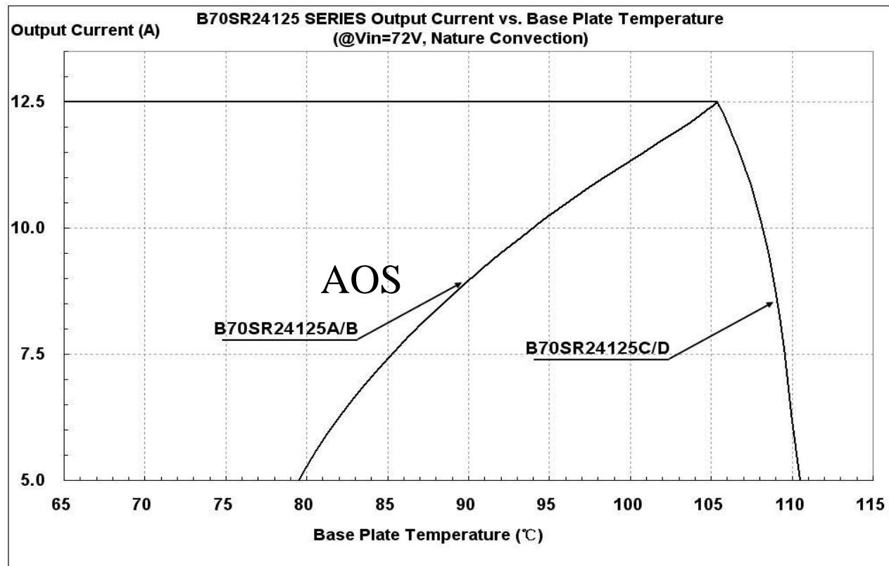
Figure 19: Output Power vs. base plate temperature @ $V_{in}=72V$
