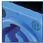
Locking area on chassis connector
