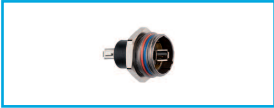
EG ● Fixed socket, female to female, nut fixing, key (W) or key (R)
