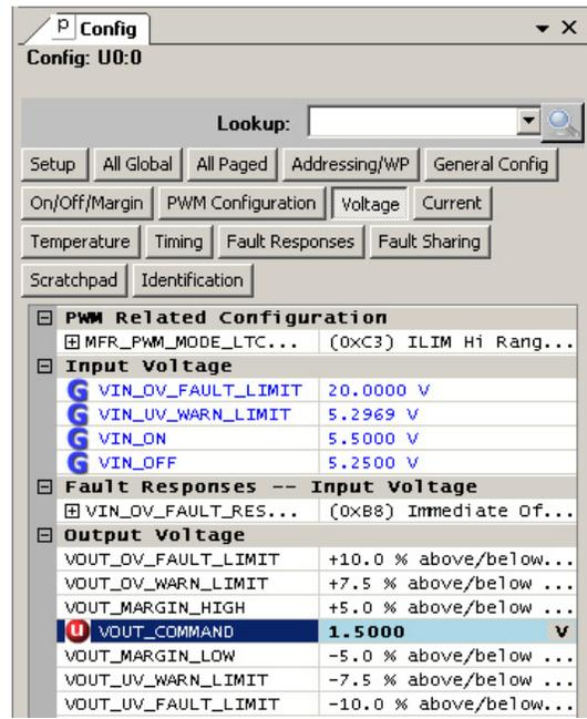
Then, click the “W” (PC to RAM) icon to write these register values to the LTM4678. After finishing this step, you will see the output voltage will change to 1.5V.
