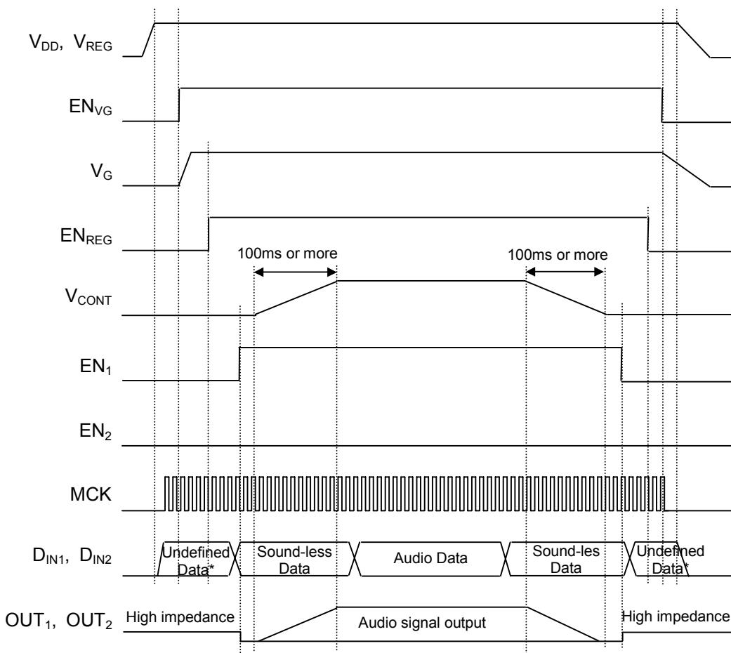
\* : Do not set  $D_{IN1}$  and  $D_{IN2}$  at "H" level before the start-up of  $V_{DD}$ .
