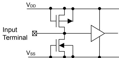
EN<sub>1</sub>, EN<sub>2</sub>, EN<sub>REG</sub>, EN<sub>VG</sub> Terminal
