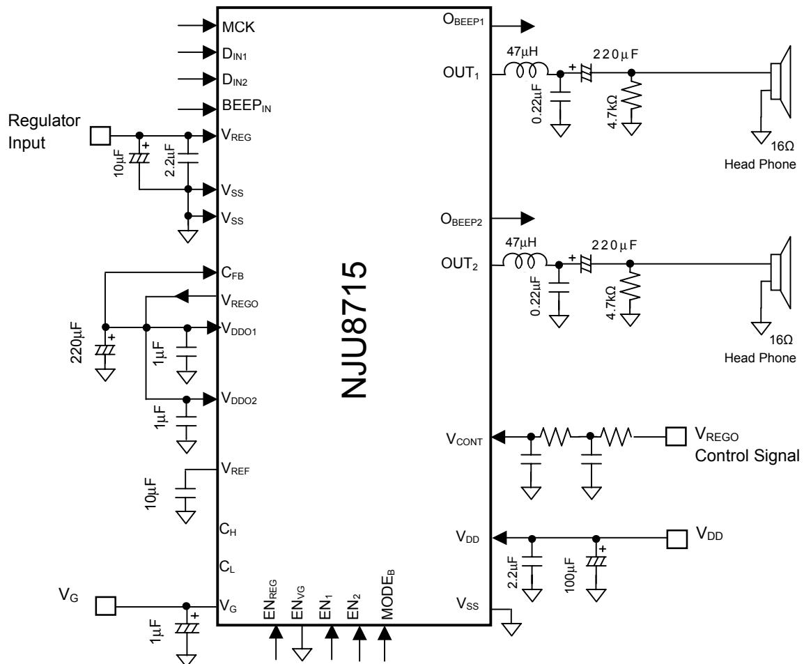
Note.7)  $C_H$  and  $C_L$  pins must be opened when  $V_G$  externally applied.
