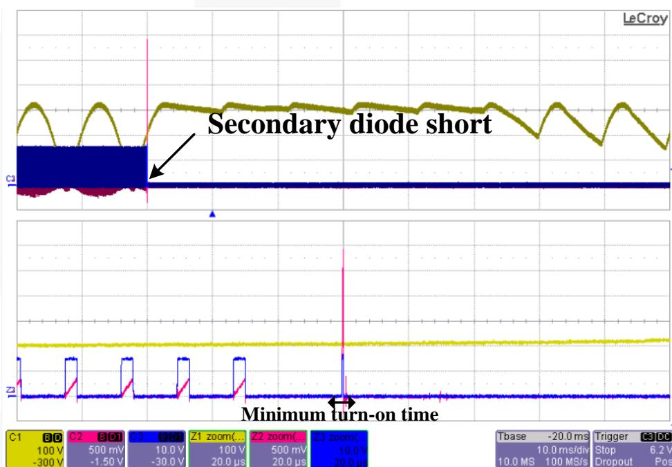
Figure 16.  $V_{IN} = 230 \text{ V}_{AC} / 50 \text{ Hz}$
