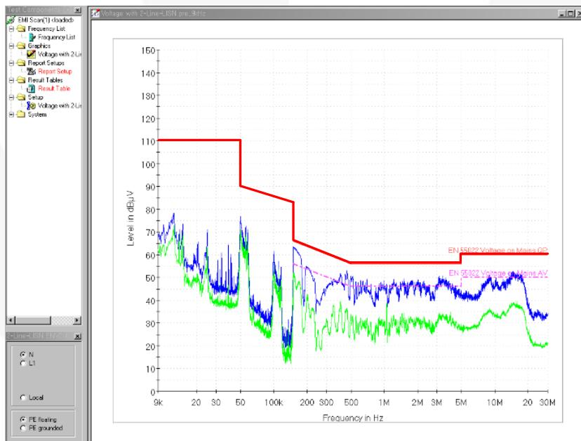
Figure 31.  $V_{IN}$  [230 V<sub>AC</sub>, Neutral ]
