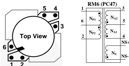
Figure 7. Transformer Bobbin Structure and Pin Configuration
