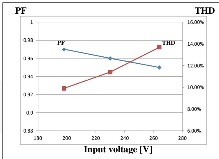
Figure 19. Power Factor & Total Harmonic Distortion
