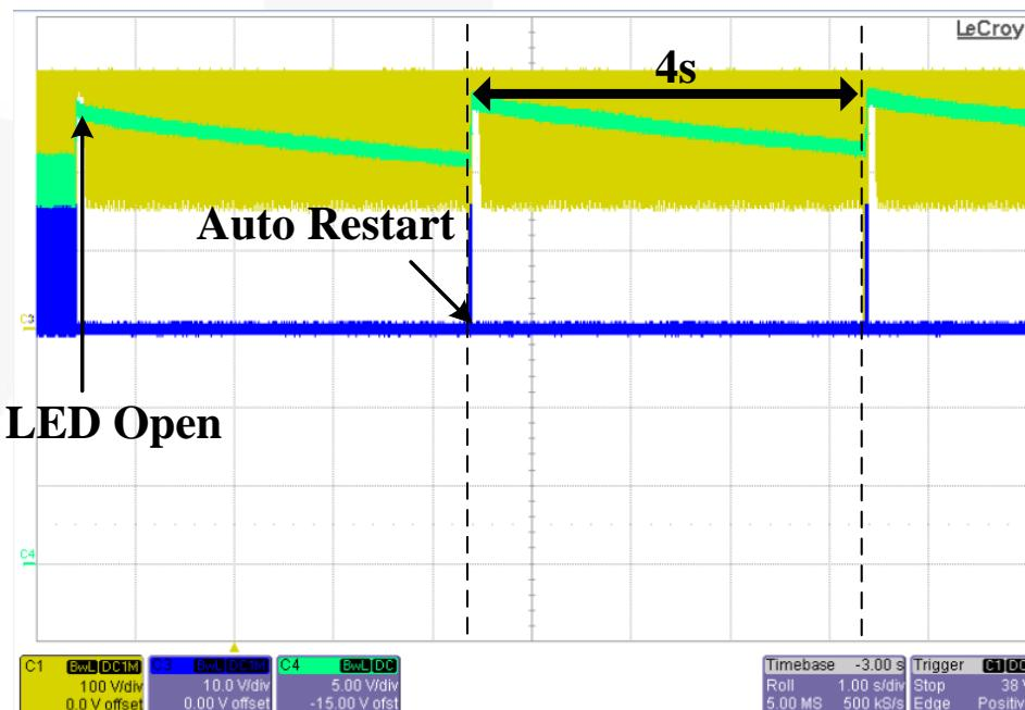
Figure 15.  $V_{IN} = 230 \text{ V}_{AC} / 50 \text{ Hz}$
